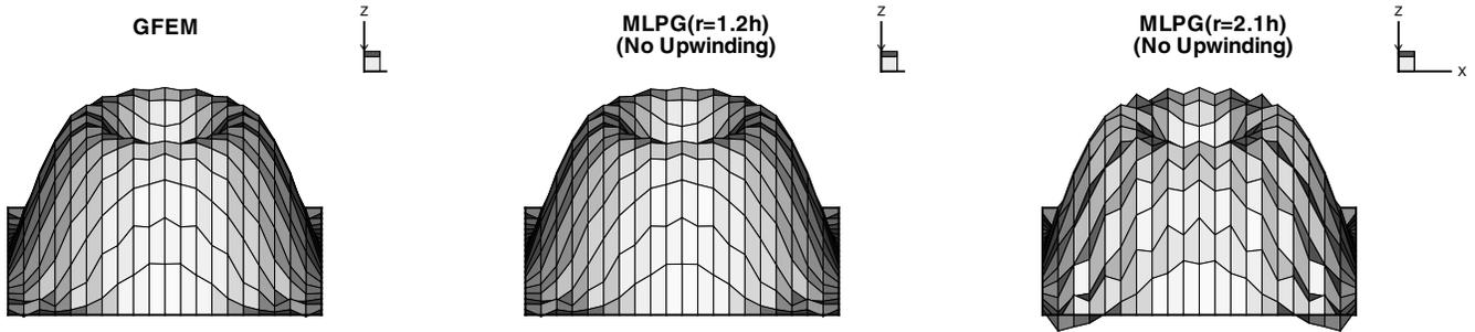
Figure 26 : Convection in a rotating flow field:  $K = 10^{-6}$  (Continued).
