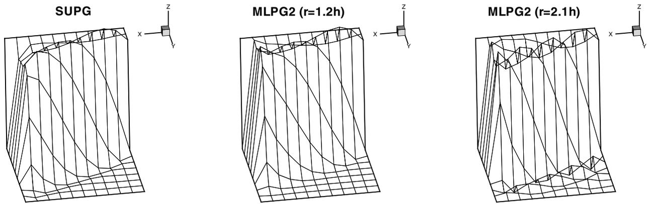
Figure 23 : Convection skew to the mesh-II:  $Pe = 10^6$  and  $\theta = \frac{\pi}{8}$ .
