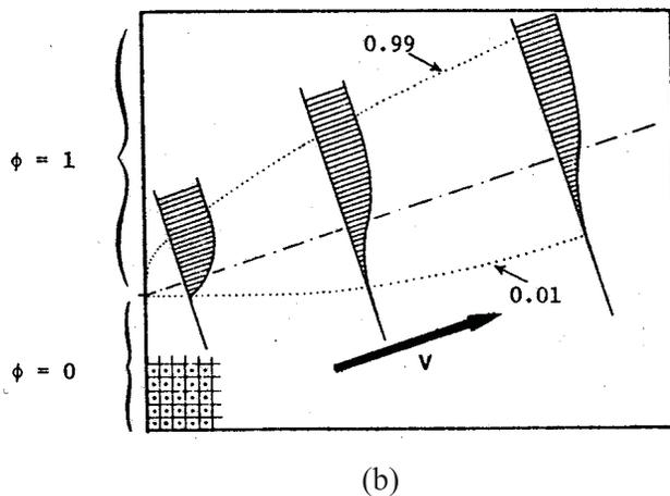
Figure 2 : Illustration of the crosswind diffusion problem with  $Pe = 100$  (from Leonard (1979)): (b) Optimal Upwinding.
