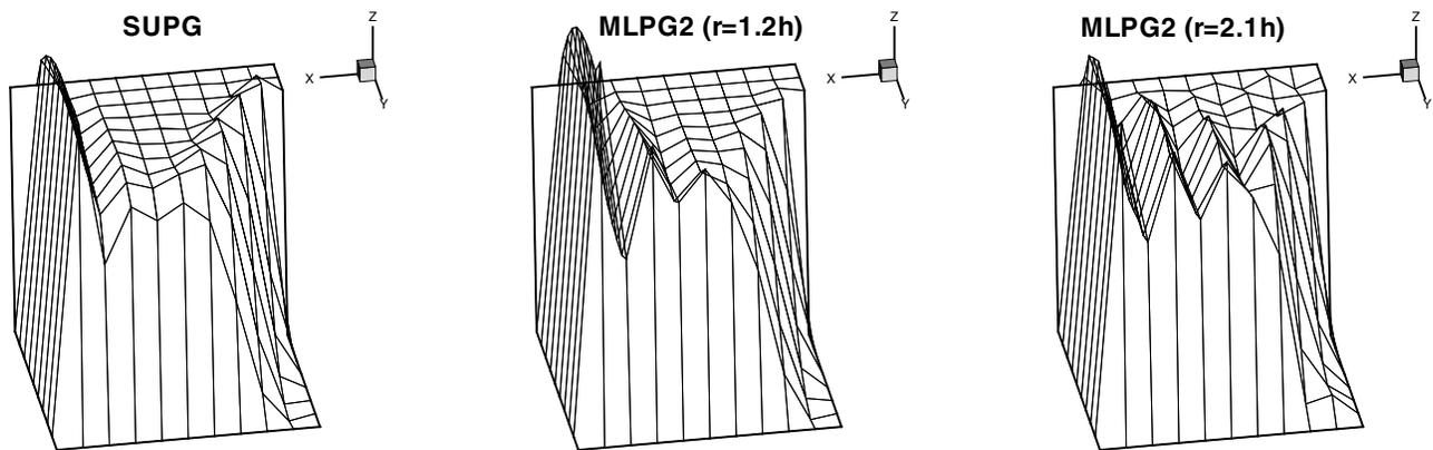
Figure 25 : Convection skew to the mesh-II:  $Pe = 10^6$  and  $\theta = \frac{3\pi}{8}$ .
