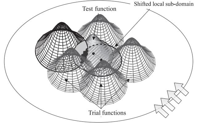
Figure 8 : MLPG Upwinding Scheme II (US-II).
