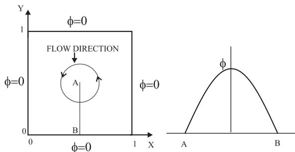
**Figure 28** : Convection in a rotating flow field: problem statement.
