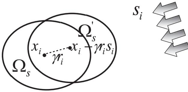
Figure 9 : MLPG Upwinding Scheme II (US-II): Specification.
