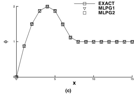
Figure 10 : Pure convection with a source term: (c) Results for MLPG1 and MLPG2.
