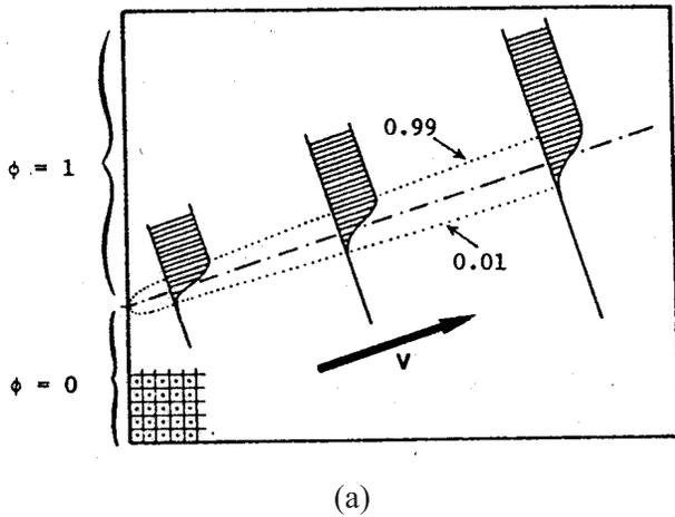
Figure 1 : Illustration of the crosswind diffusion problem with  $Pe = 100$  (from Leonard (1979)): (a) Exact.
