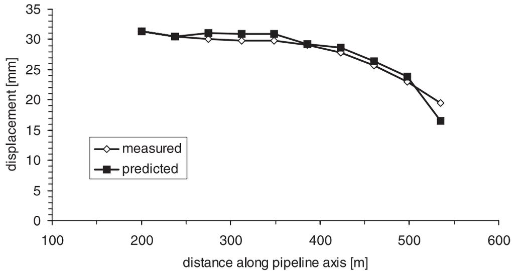
**Figure 7** : Comparison of displacements calculated by BEM soil model and by beam model from measured strain
