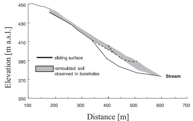
**Figure 2** : Landslide body as revealed through inclinometer measurements and boreholes
