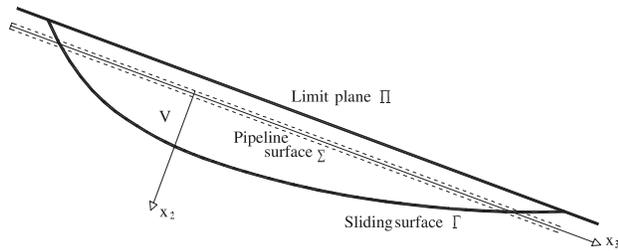
Figure 4 : Soil Volume and Boundary Model
