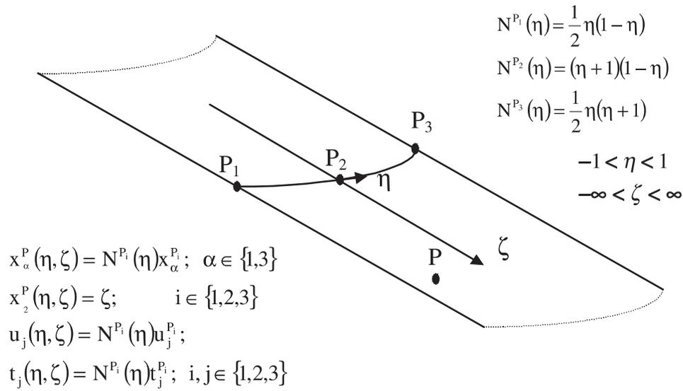
**Figure 5** : Shape functions and geometry representation on external Boundary Elements
