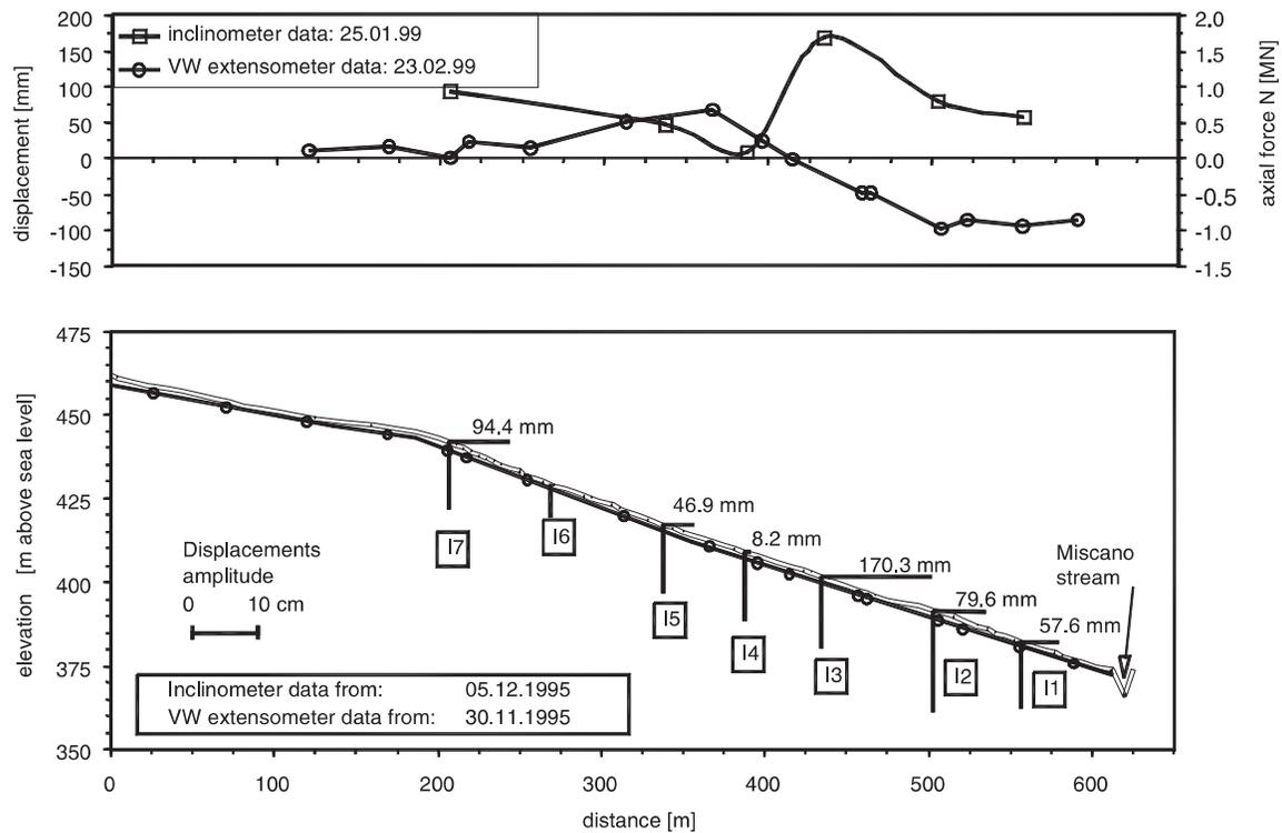
**Figure 3 :** Relevant displacements, axial force on pipeline and sliding displacements of soil
