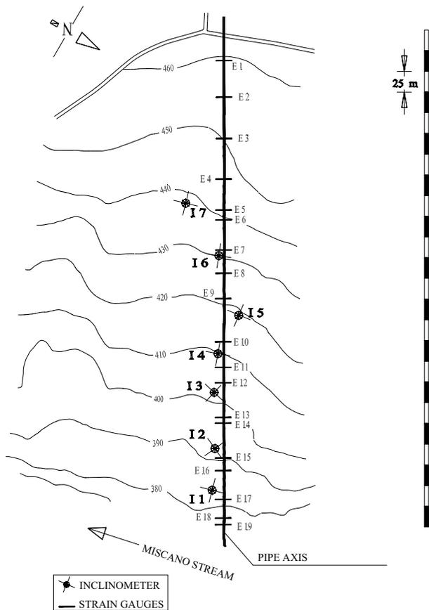
**Figure 1** : Investigated slope: instrumentation and pipeline location
