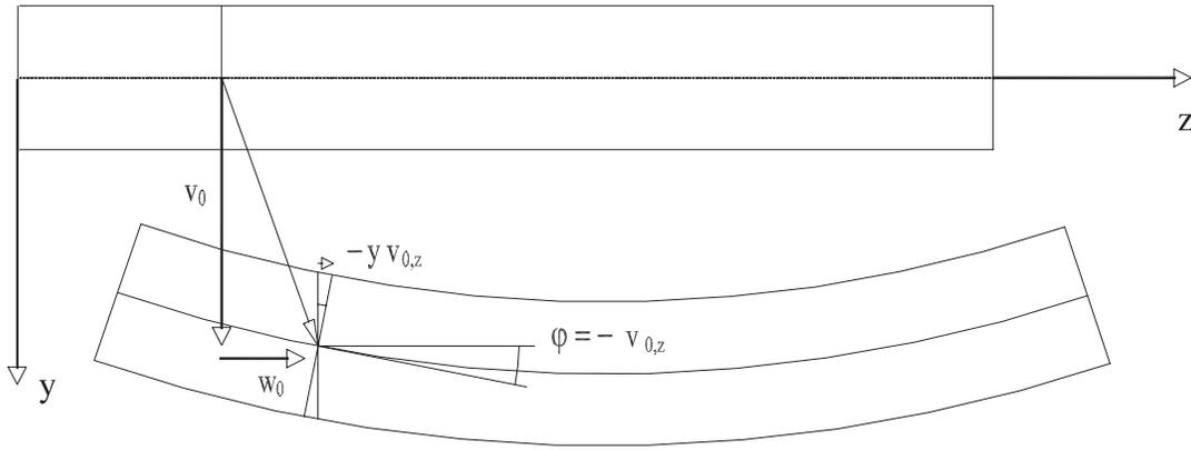
Figure 6 : Beam local coordinate system and displacements
