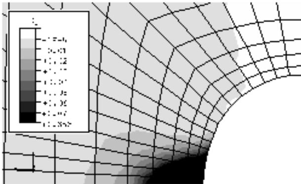
**Figure 8** : Distribution of the maximum principal damage after 3788 hours; coarser mesh r15-x6-y10-z4.
