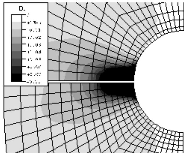
**Figure 10** : Comparison of the distribution of the maximum principal damage after 6980 hours; upper half: coarse mesh, lower half: fine mesh.
