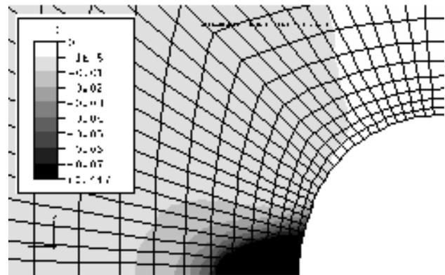
**Figure 9** : Distribution of the maximum principal damage after 3788 hours, finer mesh r24-x12-y16-z4
