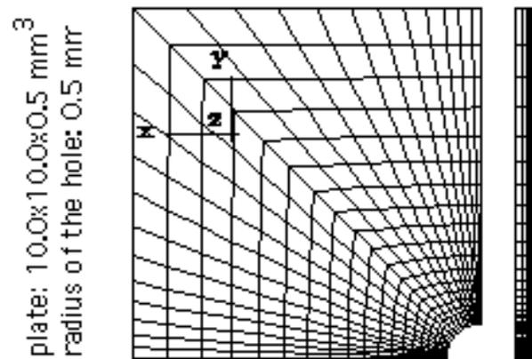
Figure 2 : FE-mesh (r20-x12-y12-z5)
