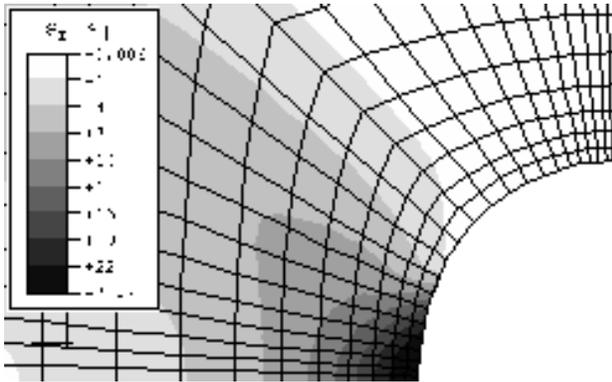
**Figure 7** : Distribution of the maximum principle strain. (Chaboche model without damage)
