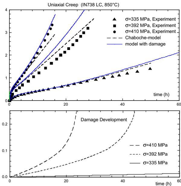
Figure 1 : Comparison of the model predictions and experiments
