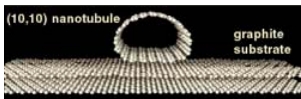
Figure 18 : Illustration of a single-shelled nanotube on graphite.
