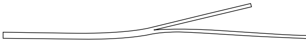
Figure 4 : Deformed shape of the lap shear joint obtained using a geometrically nonlinear analysis.
