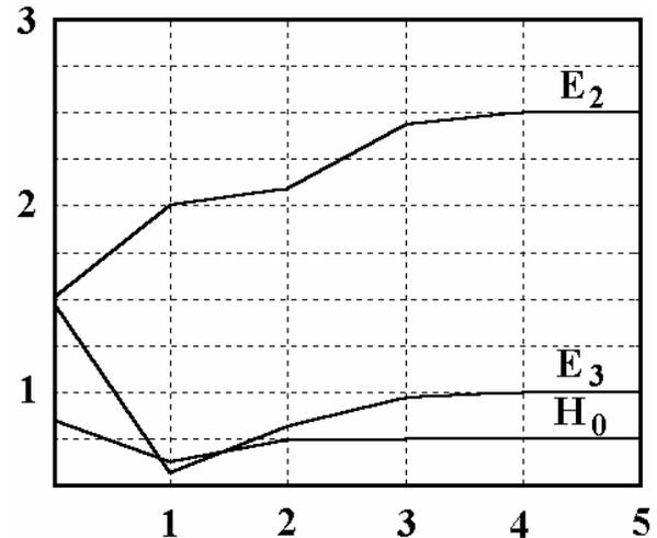
**Figure 4 :** Young moduli of the second and third layers  $E_2$  and  $E_3$  and the location of the center of the second layer as functions of the iteration index
