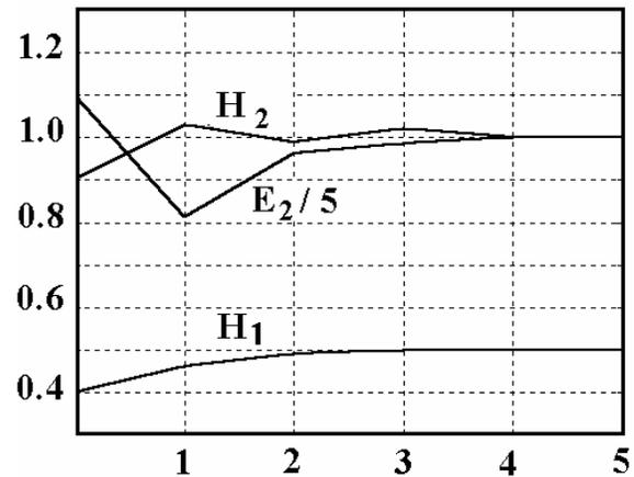
**Figure 3 :** Young modulus and boundary locations of the internal layer as a function of the iteration index
