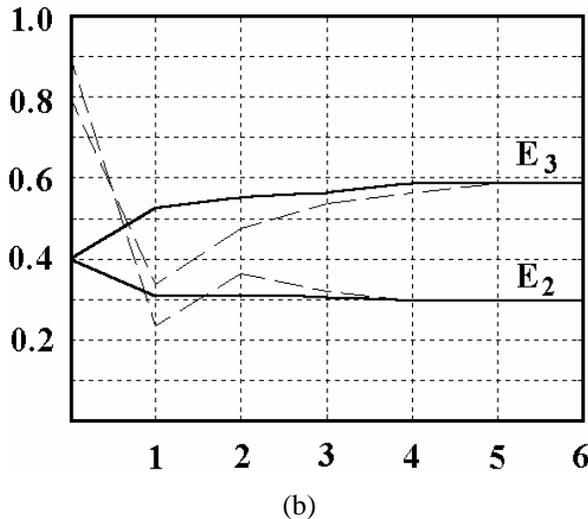
**Figure 6 :** Relative Young moduli of the second and third layers  $E_2$  and  $E_3$  as functions of the iteration index
