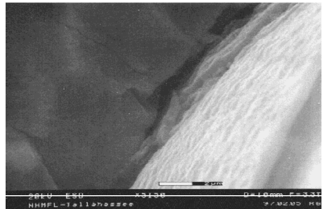
Figure 5 : Fracture surface formed during push out test on SSC-6/Timetal21s interface.
