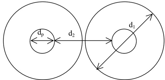
**Figure 8 :** Distance between unclustered particles
