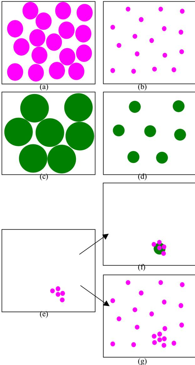
**Figure 7 :** Creation of a clustered image; (a), (b) first phase of particle laying out of clusters; (c), (d) clusters, (e), (f) and (g) second phase of clustered particles.
