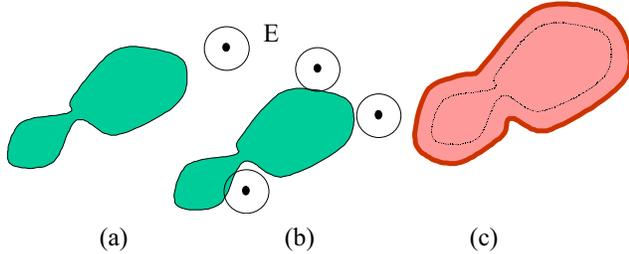
**Figure 2** : Dilation of an object by a disk. The objet A, in grey, is shown in (a) with the disk beside. The object is tested by the disk in (b), and the resulting dilated object is shown in (c).
