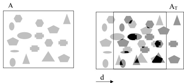
**Figure 6** : Image A and the comparison between the translated of A,  $A_T$  and A: the objects of A are in light grey and  $A_T$  objects are in dark grey. The pixels belonging to both A objects and  $A_T$  objects are in dark.
