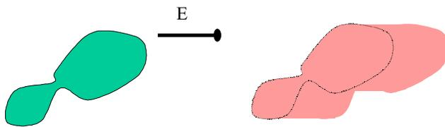
**Figure 3** : Dilation of an object by a line.
