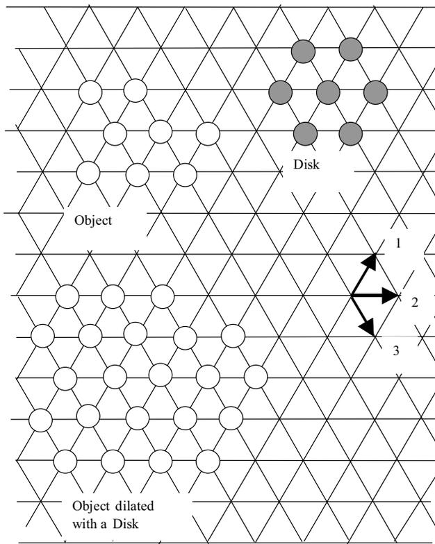
**Figure 5** : Discrete image on A hexagonal grid: the result of a dilation by a disk is shown as well as the three first directions of the hexagonal grid. The pixels are represented as circles and the lines represent the grid.
