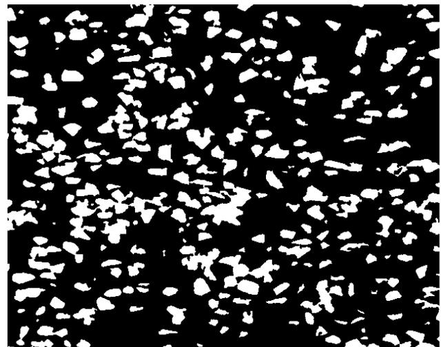
**Figure 20** : Al/SiC image after a size 1 dilation and erosion
