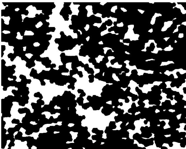
**Figure 21** : Al/SiC image after a size 6 dilation and erosion
