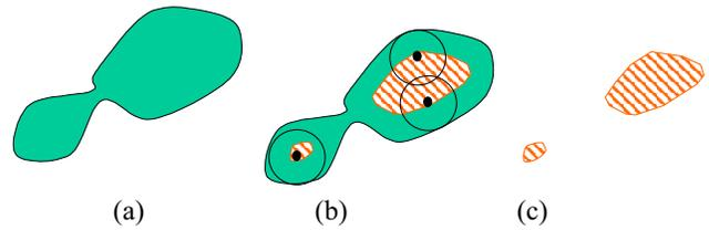
**Figure 4** : Erosion of an object by a disk. The objet A, in grey, is shown in (a). The object is tested by the disk in (b), and the resulting eroded set of two objects is shown in (c).
