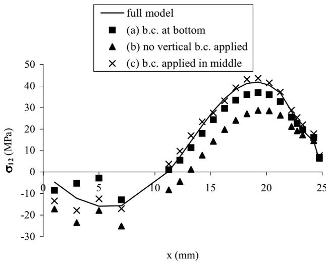
Figure 7 : Shear stress distribution through specimen width near boundary for  $\Delta a = 0.00$  mm.
