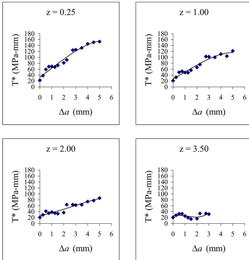
Figure 16 :  $T^*_\epsilon$  for extending crack at various through-thickness locations  $\epsilon = 3.0$  mm.
