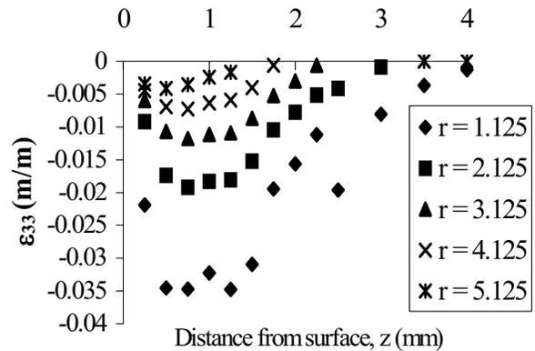
Figure 13 : Out of plane strain,  $\epsilon_{33}$  for  $\Delta a = 3.00$  mm.
