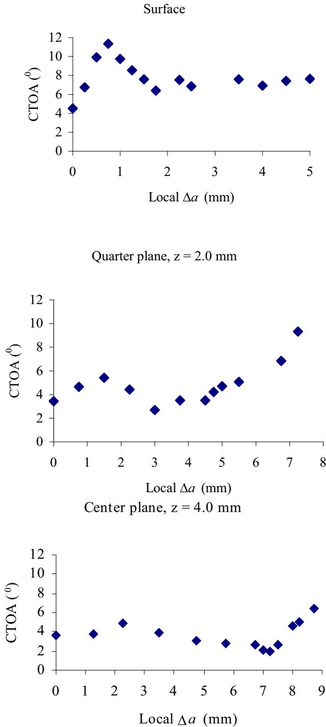
**Figure 20 :** CTOA variation through the specimen thickness.
