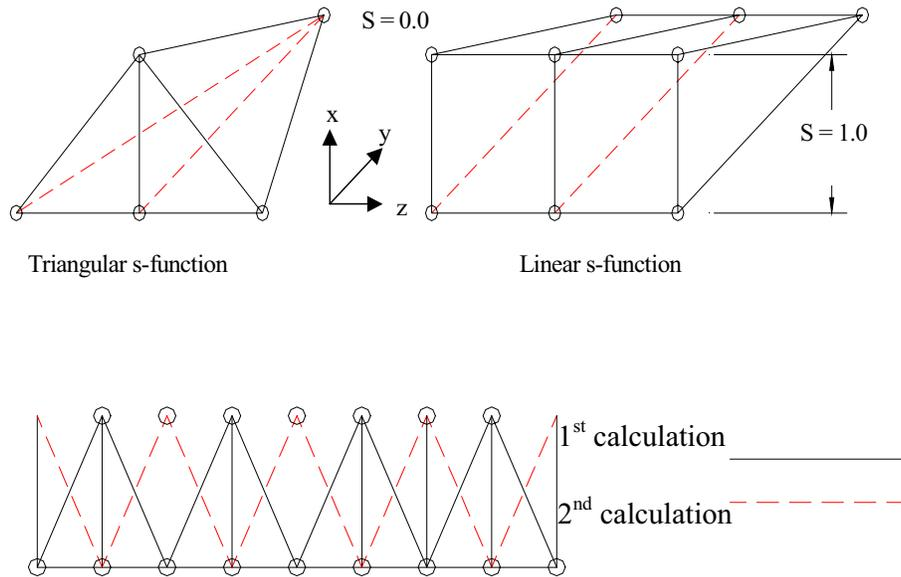
Figure 15 : Triangular and Linear s-functions with scheme to increase calculation resolution.
