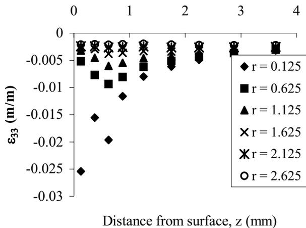
Figure 11 : Out of plane strain,  $\epsilon_{33}$  for  $\Delta a = 0.00$  mm.
