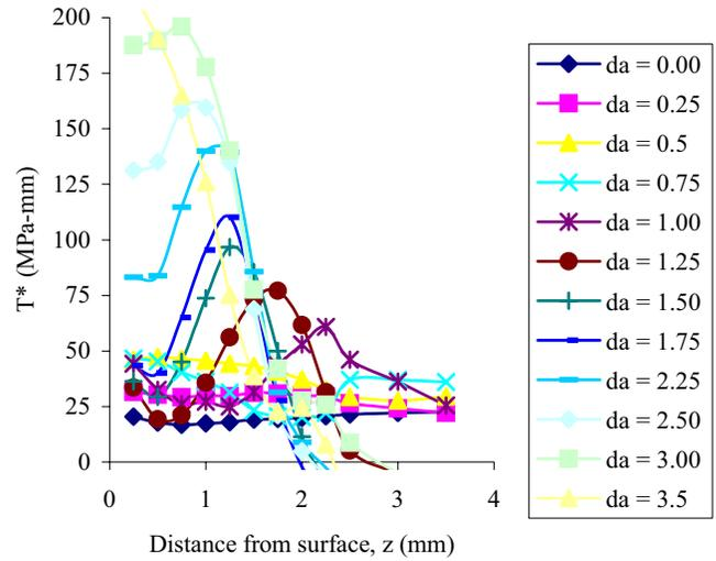
Figure 19 :  $T_{\epsilon}^*$  for an integration contour,  $\epsilon = 1.0$  mm.
