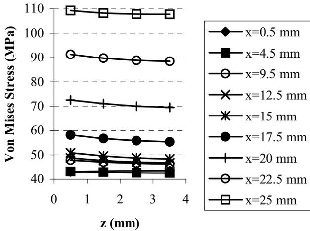
**Figure 5** : Von Mises equivalent stress through thickness at  $y=15$  mm for  $\Delta a = 1.0$  mm and  $P=3.5$  KN
