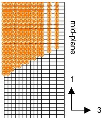
Figure 9 : Application of tunneling profile at crack tip.
