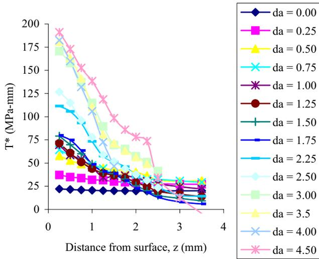
Figure 17 :  $T_{\epsilon}^*$  for an integration contour,  $\epsilon = 3.0$  mm.
