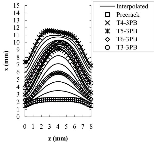
Figure 8 : Interpolated crack front profiles.
