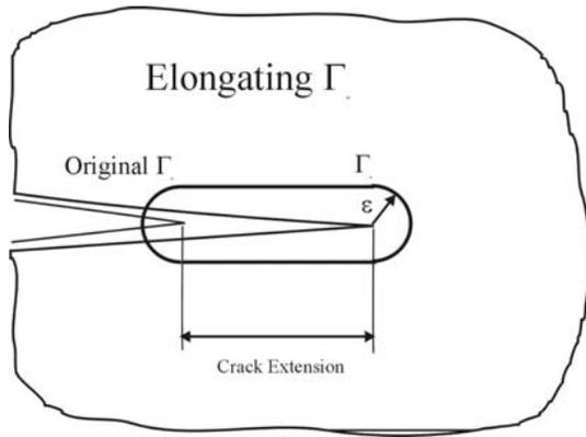
**Figure 1 :** Elongating  $\Gamma_{\epsilon}$  contour for calculation of  $T_{\epsilon}^*$
