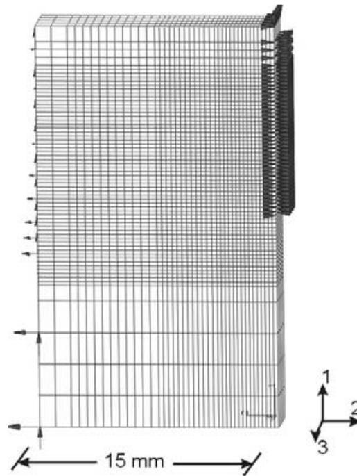
**Figure 3** : FEA model truncated at  $y=15$  mm, full height
