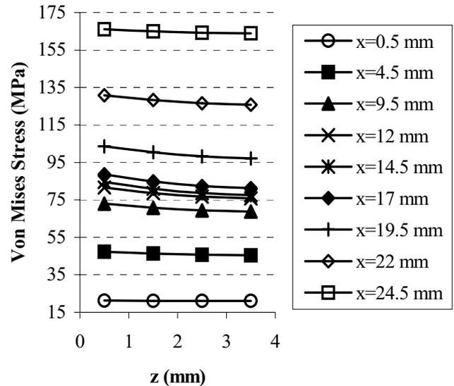
**Figure 4** : Von Mises equivalent stress through thickness at  $y = 9.5$  mm for  $\Delta a = 1.0$  mm and  $P=3.5$  KN.
