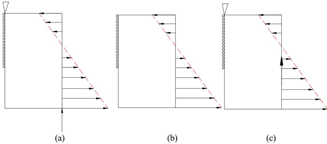
Figure 6 : Transverse displacement boundary conditions applied at truncation boundary.
