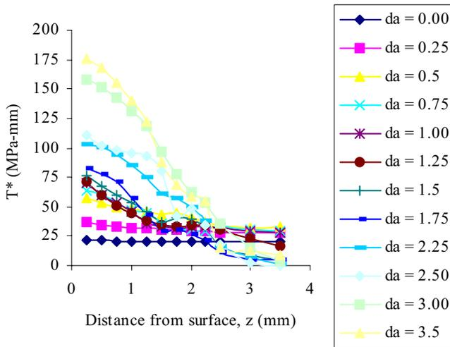
Figure 18 :  $T_{\epsilon}^*$  for an integration contour,  $\epsilon = 2.0$  mm.
