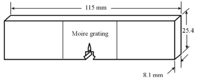
**Figure 2 :** Three-point bend specimen with moir grating
