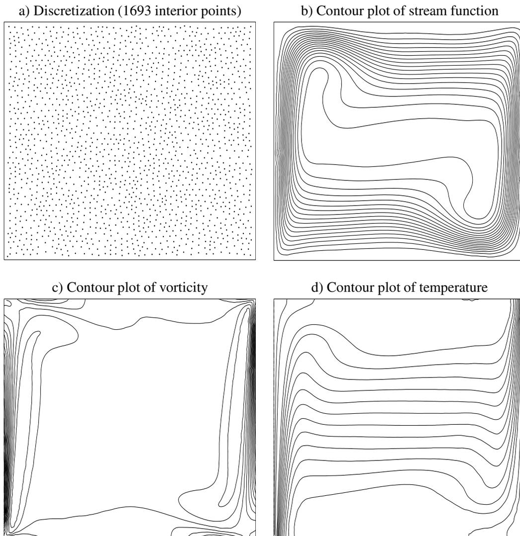
**Figure 10** : Natural convection flow, 1693 interior points,  $Ra = 1.e6$ : discretization and some contour plots.
