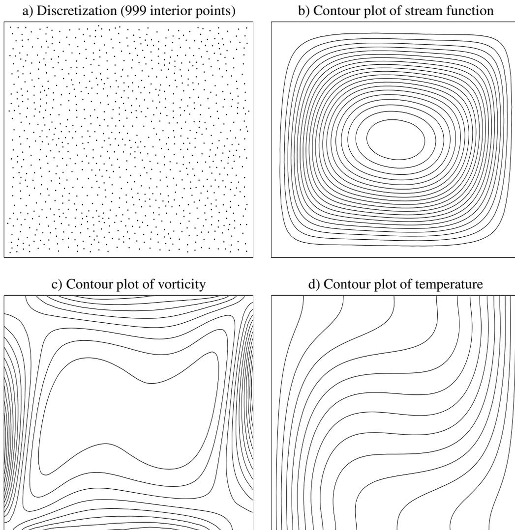
**Figure 8** : Natural convection flow, 999 interior points,  $Ra = 1.e4$ : discretization and some contour plots.
