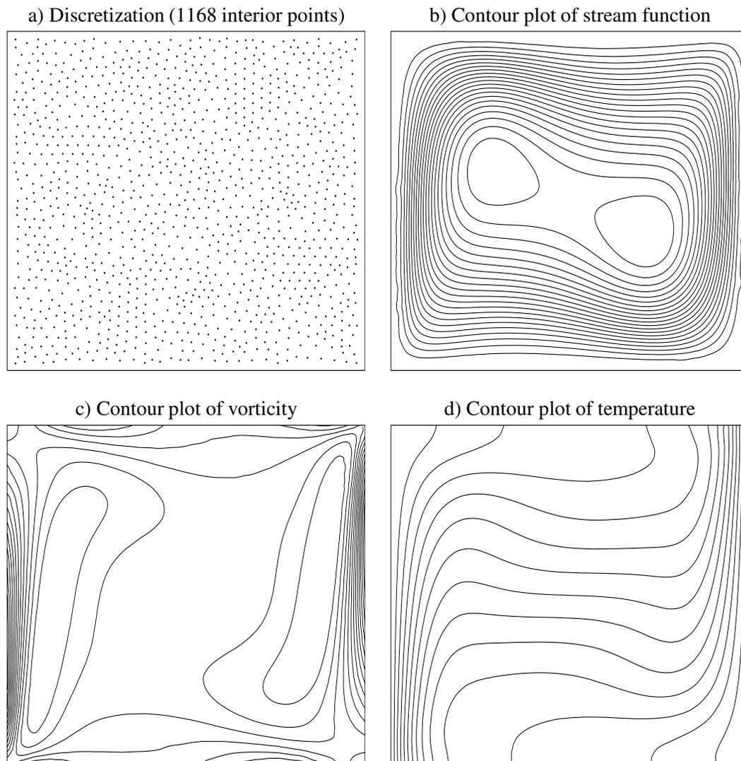
**Figure 9** : Natural convection flow, 1168 interior points,  $Ra = 1.e5$ : discretization and some contour plots.
