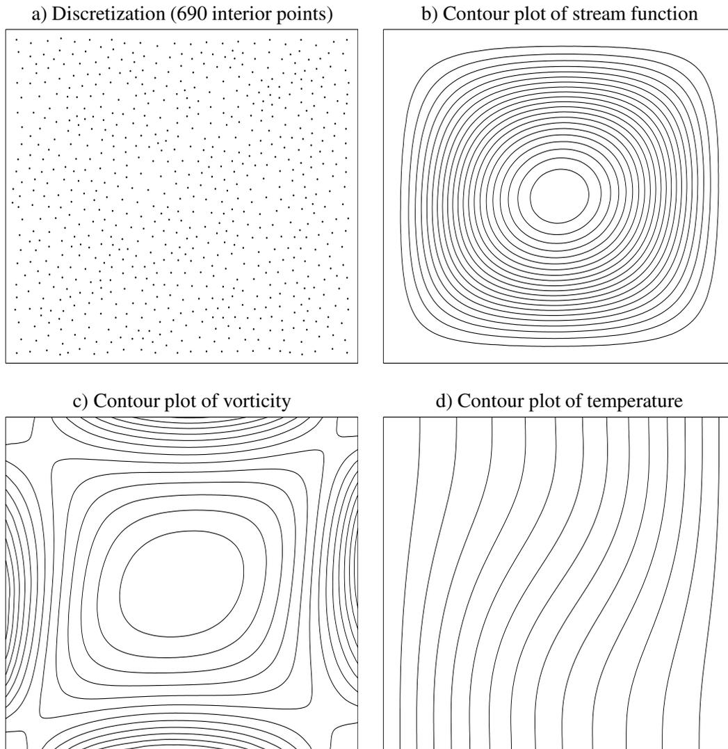
**Figure 7** : Natural convection flow, 690 interior points,  $Ra = 1.e3$ : discretization and some contour plots.
