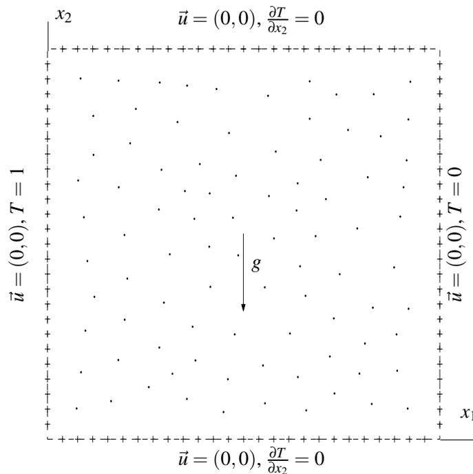
**Figure 6** : Natural convection flow in a square cavity: geometry definition, boundary conditions and discretization. Legends +: boundary point and .: interior point. The problem domain is simply represented by a set of scattered points.
