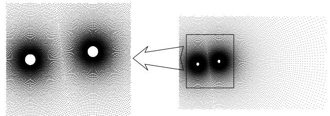
**Figure 9 :** Node distribution for the flow around two staggered circular cylinders
