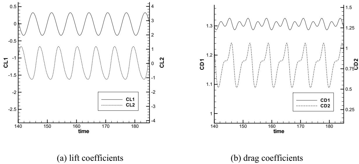
**Figure 11 :** Time history of drag and lift coefficients for the flow around two staggered circular cylinders at  $Re = 100$
