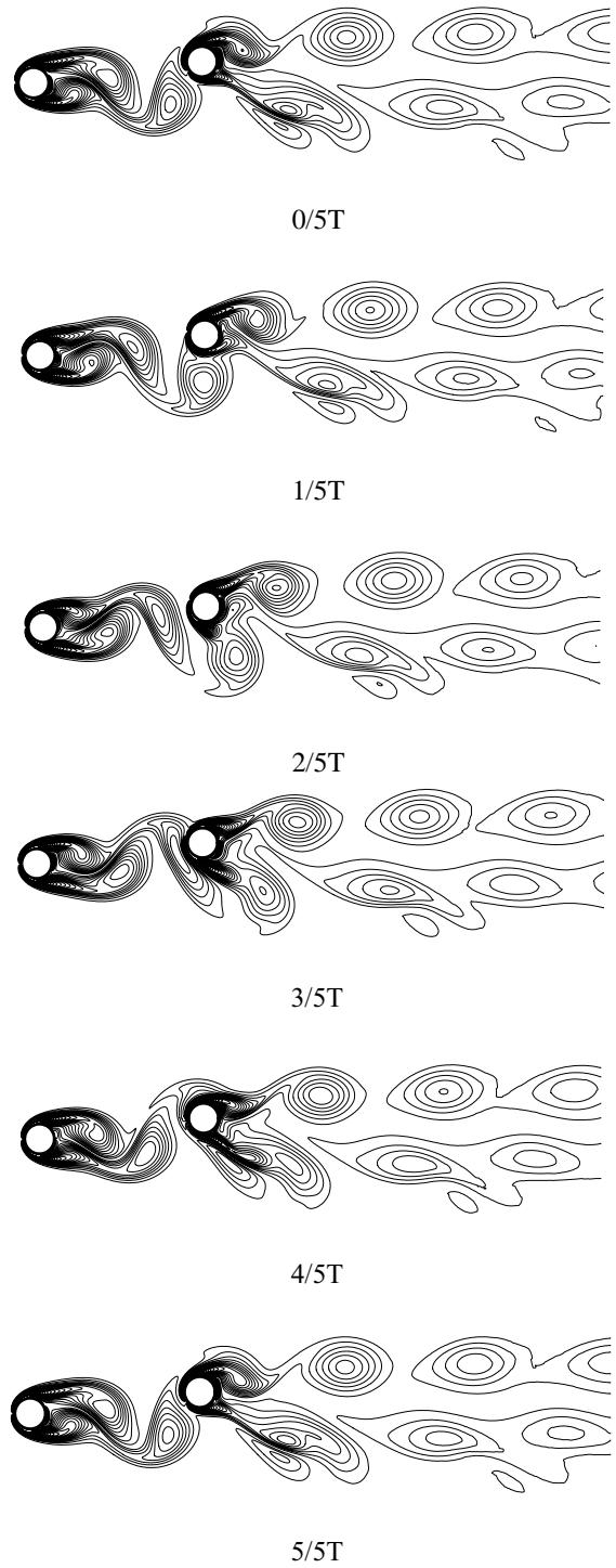
**Figure 10 :** Vorticity contours for the flow around two staggered circular cylinders at  $Re = 100$  in one complete circle
