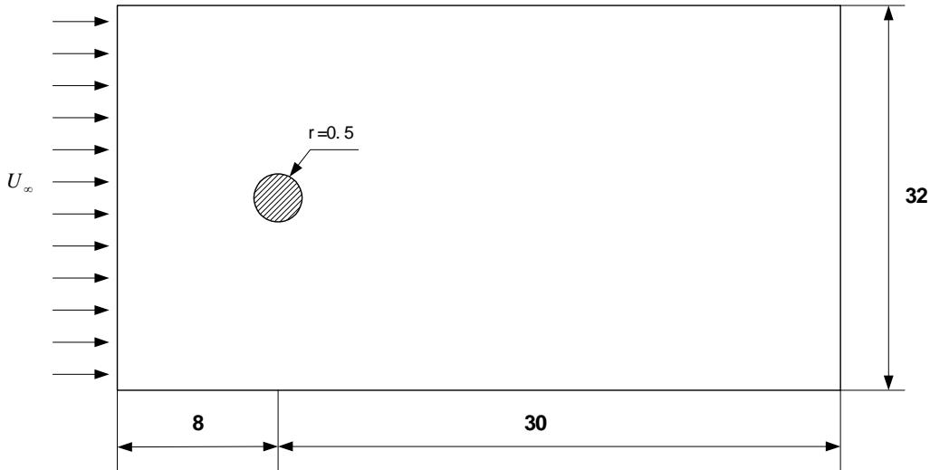
**Figure 4 :** Configuration of flow around one isolated cylinder
