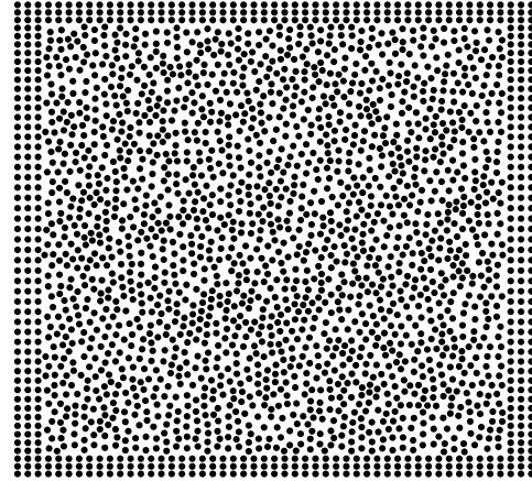
Figure 2 : Orthogonal boundary grids and interior random knots
