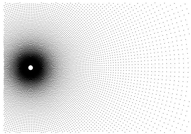
**Figure 5 :** Node distribution for flow past one isolated circular cylinder
