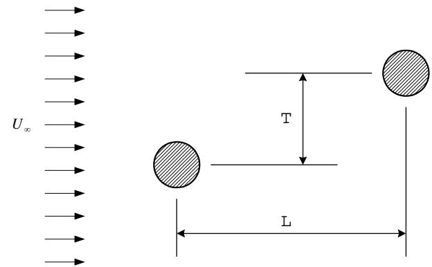
**Figure 8 :** Geometrical description of flow past a pair of cylinders
