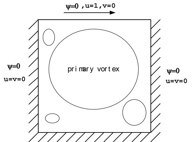
Figure 1 : Lid-driven flow in a square cavity
