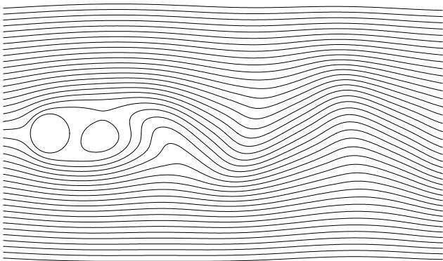
**Figure 6 :** Streamlines and vorticity contours for  $Re = 100$
