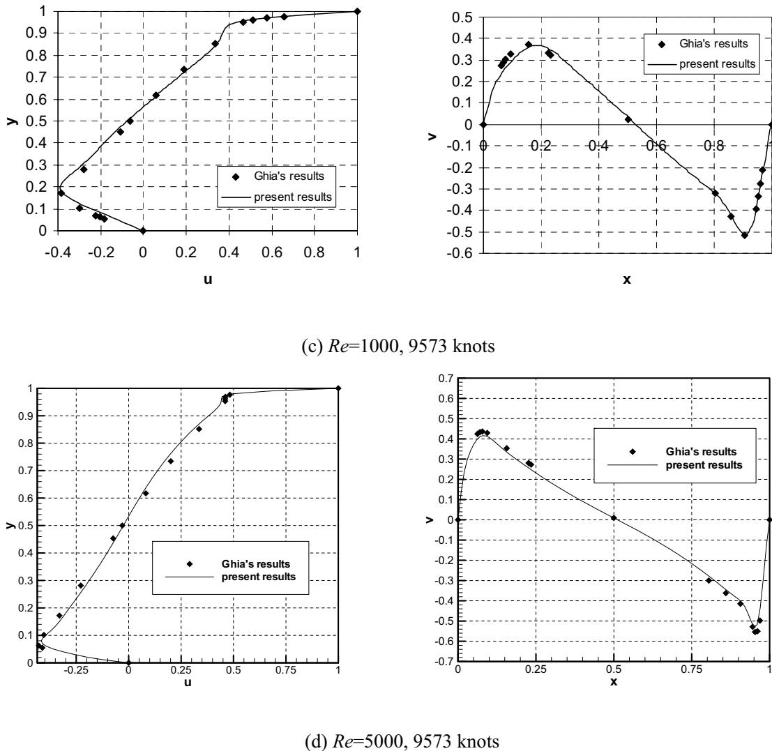
**Figure 3 :** U (left) and V (right) velocity profiles along vertical and horizontal central lines
