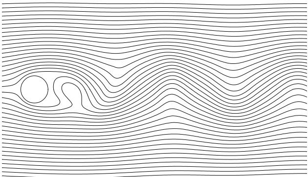
**Figure 7 :** Streamlines and vorticity contours for  $Re = 200$
