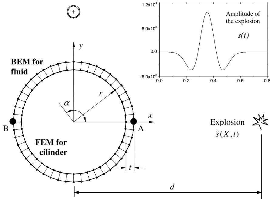
Figure 2 : Submerged cylinder subjected to an external explosion.
