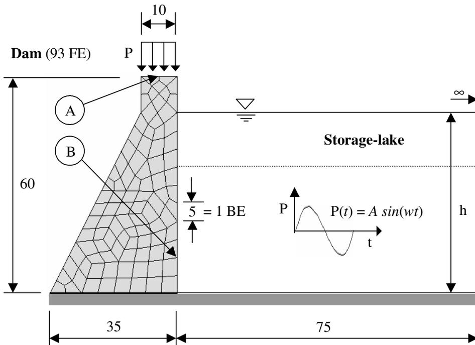
Figure 5 : Dam retaining the water of a semi-infinite storage-lake.
