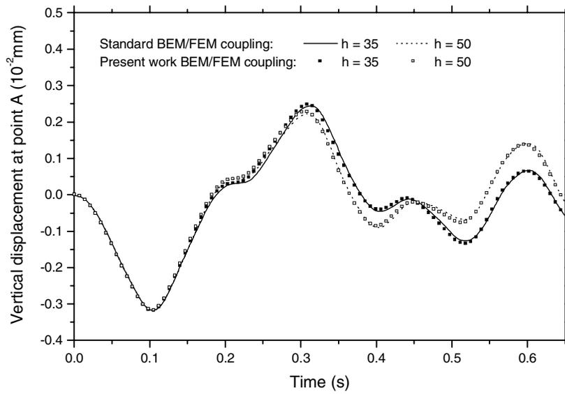
Figure 6 : Vertical displacement at point A: influence of the water level.
