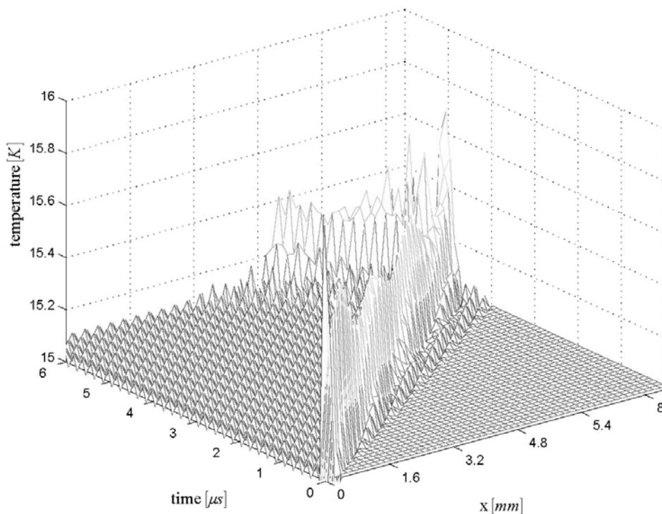
**Figure 3 :** Heat conduction in NaF, type II, cG approximation. Heat propagates as a wave. Oscillations enforce a stabilization.
