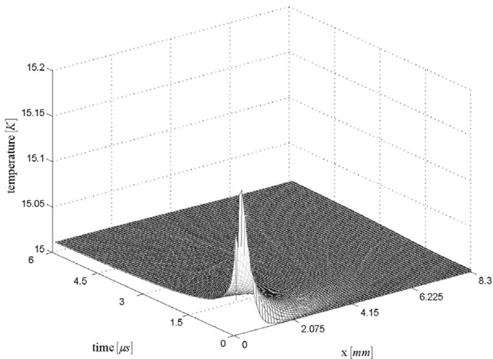
**Figure 2 :** Heat conduction in NaF, type I, dG approximation. Heat does not propagate as a wave.
