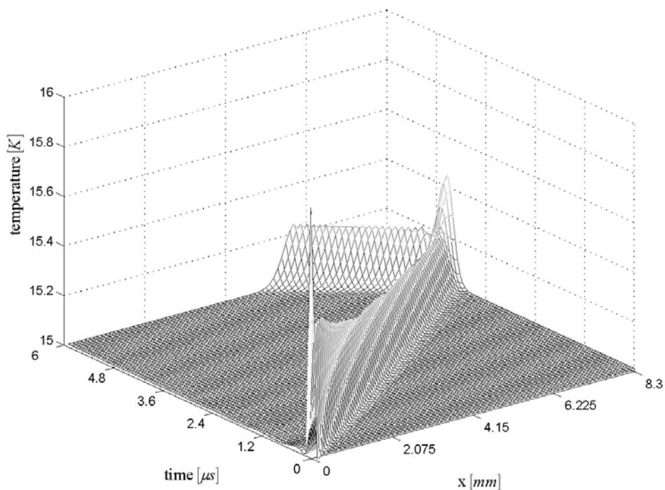
**Figure 4** : Type II, approximated by cG and stabilized with a Streamline-Upwind-Method, does not involve energy dissipation.
