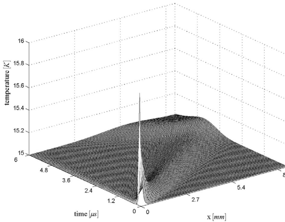
**Figure 6 :** Heat conduction in NaF, type III, cG approximation, permits propagation of heat as a diffusive wave. This heat flow is perfectly stable.
