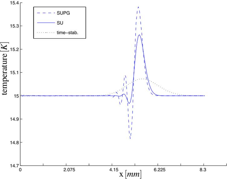
Figure 13 : Stabilized problem: Temperature plotted versus position at time  $t = 3\mu$  s. Again it can be seen that the SUPG-solution oscillates and that the time-stabilized wave is damped too much whereas the SU-solution seems to be suitable.
