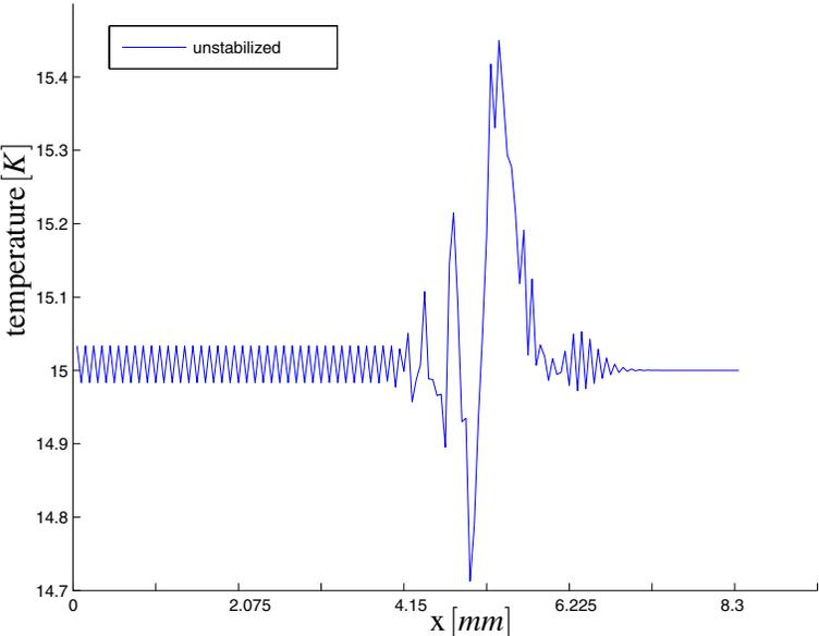
Figure 12 : Temperature is now plotted versus position in the unstabilized case at time  $t = 3\mu$  s. Oscillations are again clearly visible.
