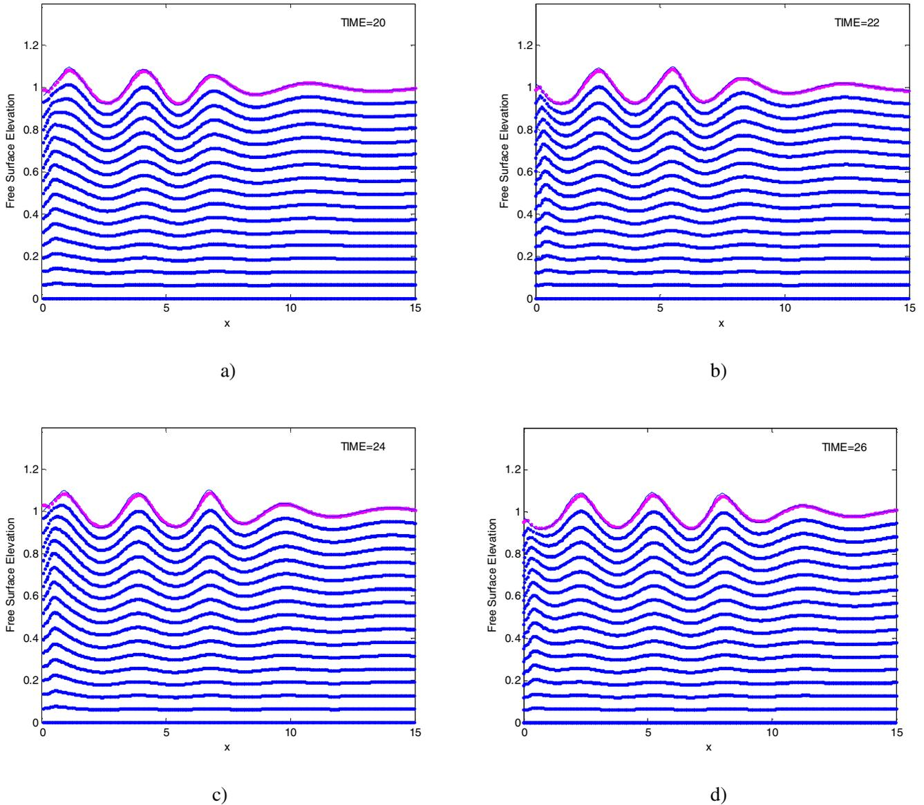
**Figure 8** : Comparison of wave profiles obtained by MLPG\_R and FEM for  $S_0=0.05$  and  $\omega=1.45$ . (Dots: node configuration obtained by MLPG\_R; solid line: the free surface obtained by FEM)
