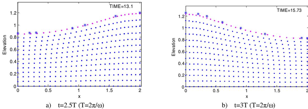
**Figure 11 :** Configurations of nodes at two instants for  $X_0=0.0186$  and  $\omega/\omega_{n0} \approx 0.999$  (\*: experimental data from Okamoto and Kawahara (1990))
