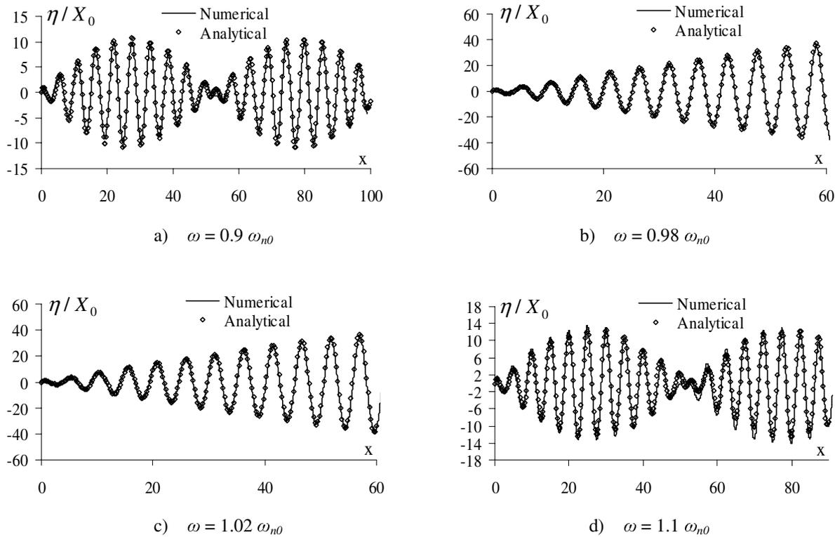
**Figure 10 :** Time histories of sloshing waves at  $x=0$  for different frequencies (the analytical solution from Faltinsen (1978))
