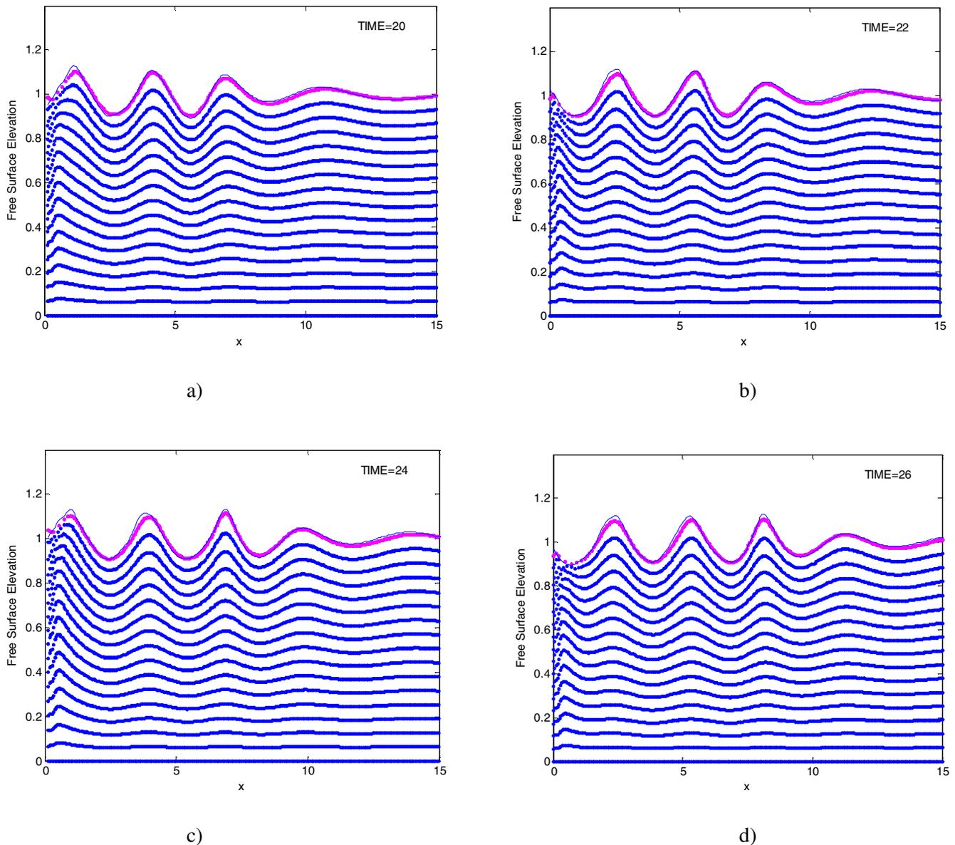
**Figure 9** : Comparison of wave profiles obtained by MLPG\_R and FEM for  $S_0=0.064$  and  $\omega=1.45$ . (Dots: node configuration obtained by MLPG\_R; solid line: the free surface obtained by FEM)
