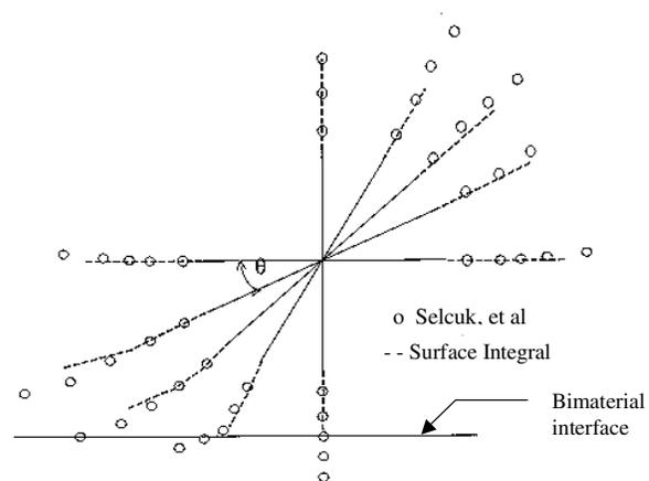
**Figure 8 :** Crack growth trajectories for  $E_2/E_1 = 5$ .
