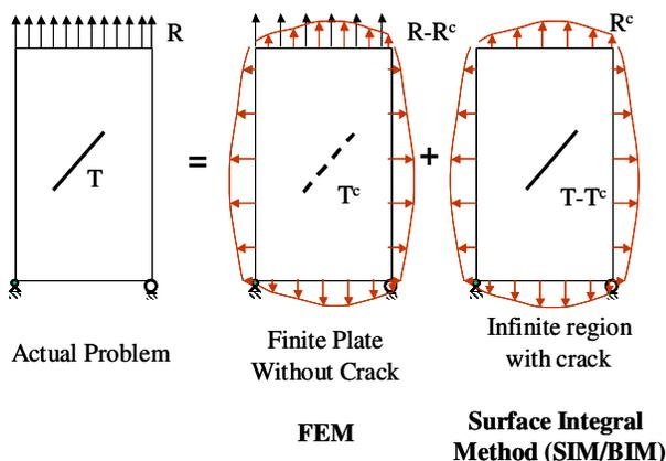
Figure 4 : Schematic of linear superposition.
