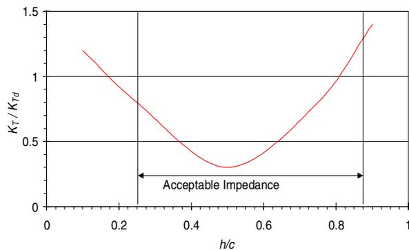
**Figure 13 :** Effect of wire placement on impedance and initiation of delamination.
