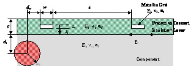
Figure 3 : Definition of crack sensor system (cross section).
