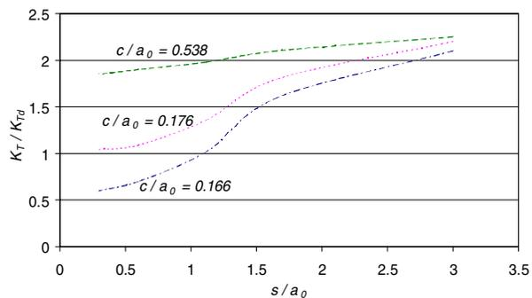
**Figure 12 :** Effect of coating thickness and wire spacing on delamination.
