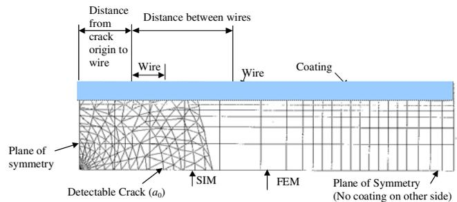
**Figure 11** : Hybrid Finite element mesh (FEM) and Surface integral mesh (SIM) to predict wired coating failure. Wires break as the crack in the part propagates.
