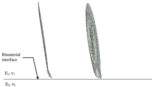
**Figure 9** : Growth of a pressurized crack towards an interface (2 views).  $E_2/E_1 = 5$ ,  $\nu_1 = \nu_2 = 0.3$  and  $\theta = 60$ .
