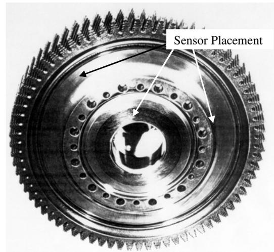
**Figure 1** : Component schematic and sensor placement location.
