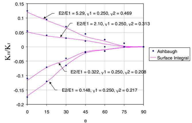
**Figure 6 :** Comparison of results for a 3D rectangular crack near an interface to a 2D plane strain solution. ( $e/a = 0.4$ , aspect ratio of crack = 10).
