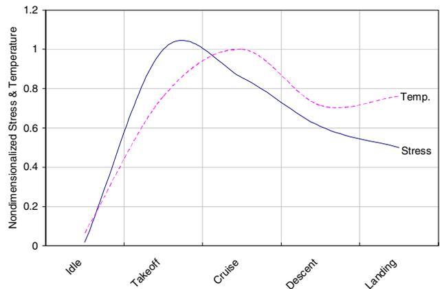
Figure 2 : Idealized loading and thermal sequence.
