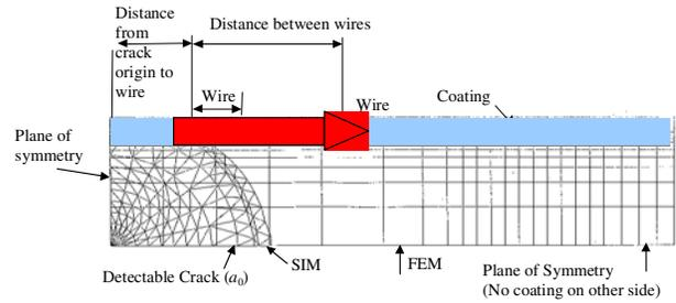
**Figure 10** : Hybrid Finite element mesh (FEM) and Surface integral mesh (SIM) to predict wired coating failure.
