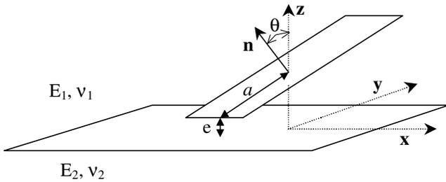
**Figure 5 :** Definition of a 3D rectangular crack near a planar interface.
