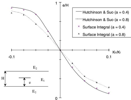
**Figure 7 :** Stress intensity factor ratio versus crack depth for a crack in a layered material.
