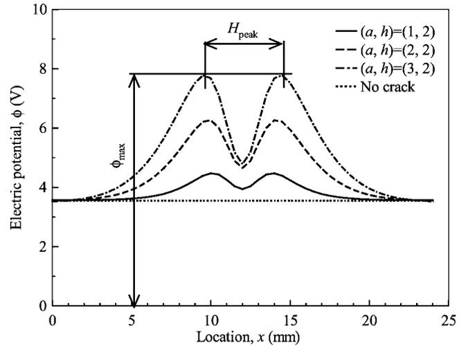
**Figure 2 :** Effect of crack length  $a$  on electric potential distributions for a plate with a single crack
