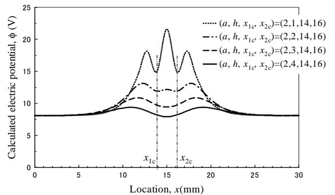
**Figure 6 :** Effect of crack depth  $h$  on electric potential distributions for a plate having plural cracks with length of  $a=2$  located at  $x_{1c}=14$  and  $x_{2c}=16$ .
