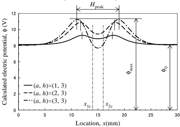
**Figure 5 :** Effect of crack length  $a$  on electric potential distributions for a plate having plural cracks with depth of  $h=3$  located at  $x_{1c}=14$  and  $x_{2c}=16$ .
