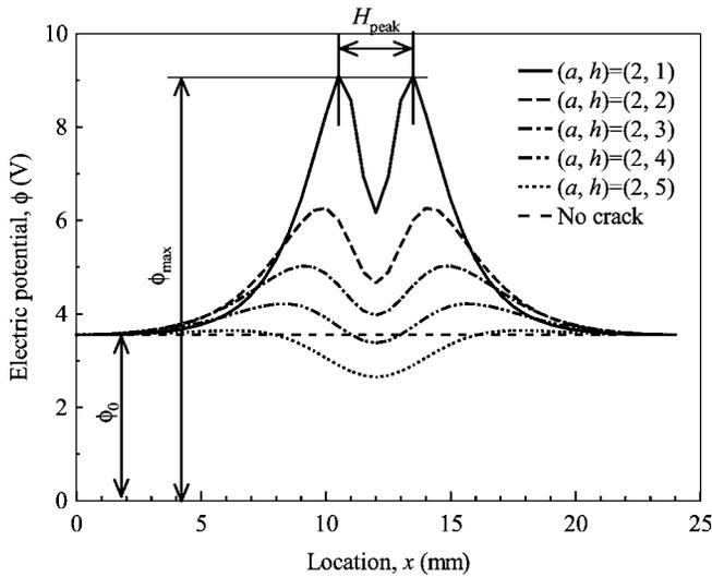
**Figure 3 :** Effect of crack depth  $h$  on electric potential distributions for a plate with a single crack
