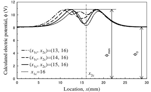
**Figure 4 :** Effect of distance between cracks ( $x_{2c} - x_{1c}$ ) on electric potential distributions for a plate with plural cracks with length of  $a=2$  and depth of  $h=3$ .
