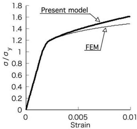
Figure 8: Macroscopic stress-strain relation without the strain gradient effect ( $c = 0$ )
