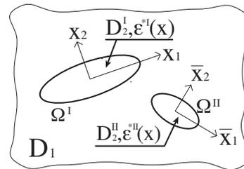
Figure 2: Multi-particle model.
