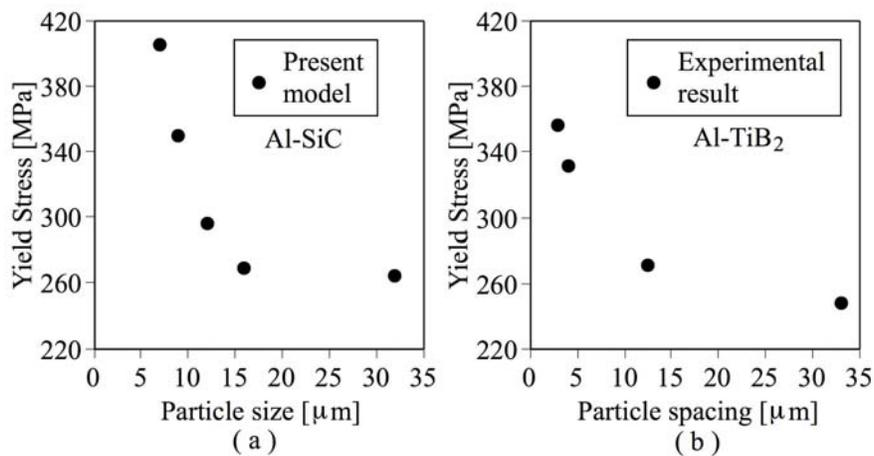
Figure 10: 0.2 % offset yield stress. (a) Results of the present study (b) Experimental results
