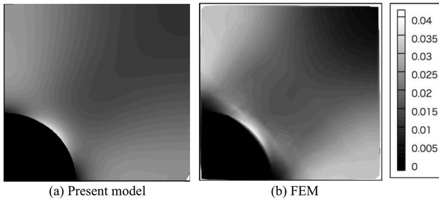
Figure 7: Strain distribution without the strain gradient effect ( $c = 0$ ) when the macroscopic strain is 0.015 (a) Present model (b) conventional FEM.
