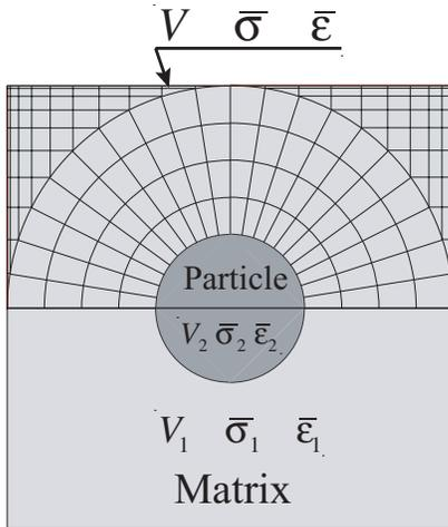
Figure 4: A unit cell in the present model
