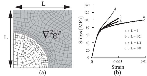
Figure 1: Previous study (a):Composite model with fine mesh (b):Macroscopic stress-strain curve for uniaxial tensile loading obtained from the gradient plasticity
