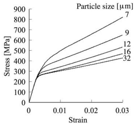
Figure 9: Stress-strain curve depending on particle size ( $c = -0.01$ )
