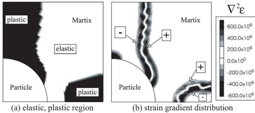
Figure 11: Plasticity and strain distribution domain when the macroscopic strain is 0.002 and coefficient  $c$  is zero.
