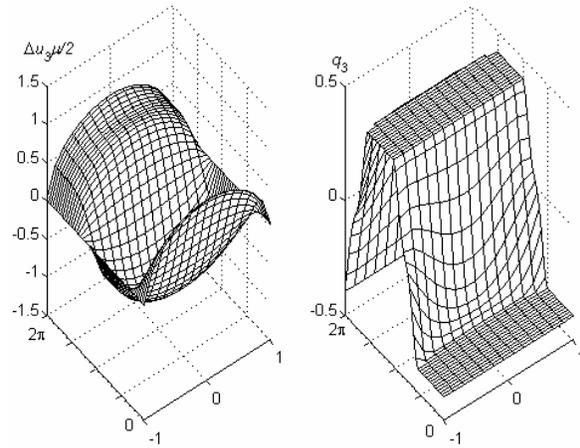
Figure 9: Crack opening and friction contact force for  $k_2 = 0.25$  and  $k_\tau = 0.4$ .
