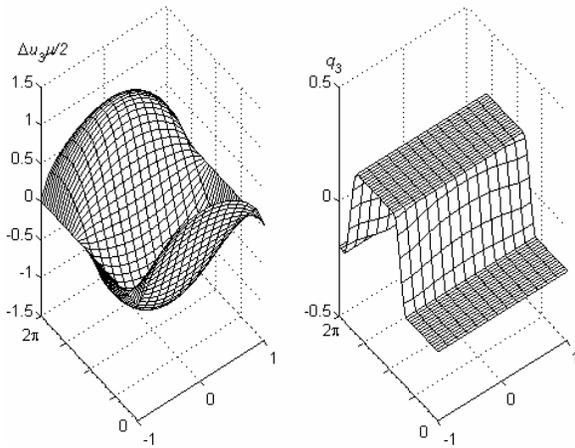
Figure 10: Crack opening and friction contact force for  $k_2 = 1.0$  and  $k_\tau = 0.2$ .
