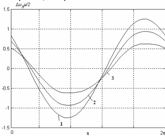
Figure 4: Crack opening  $k_2 = 1.0$ :  $1 - k_\tau = 0$ ,  $2 - k_\tau = 0.2$ ,  $3 - k_\tau = 0.4$ .
