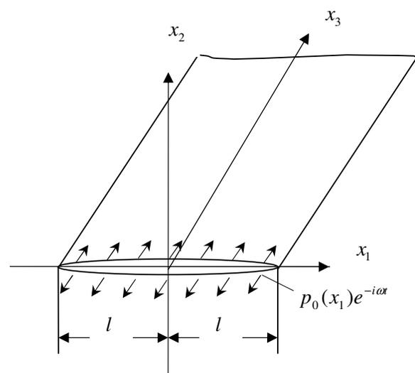
Figure 1: Finite crack under antiplane deformation
