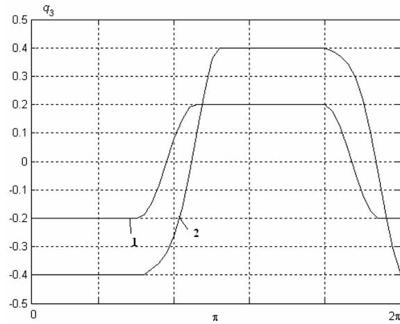
Figure 3: Friction contact force for  $k_2 = 0.25$ :  $1 - k_\tau = 0.2$ ,  $2 - k_\tau = 0.4$ .
