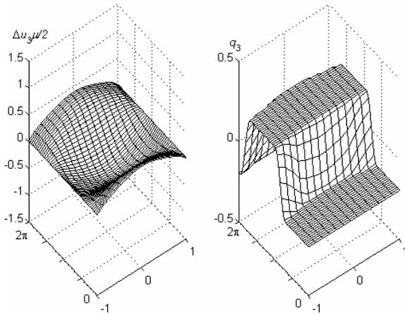
Figure 12: Crack opening and friction contact force for  $k_2 = 1.75$  and  $k_\tau = 0.2$ .
