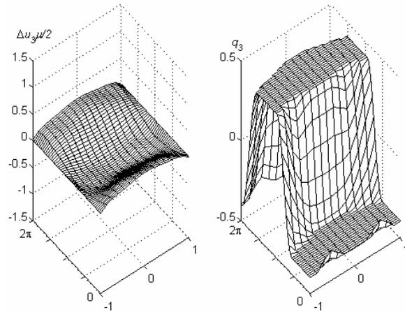
Figure 13: Crack opening and friction contact force for  $k_2 = 1.0$  and  $k_\tau = 0.4$ .
