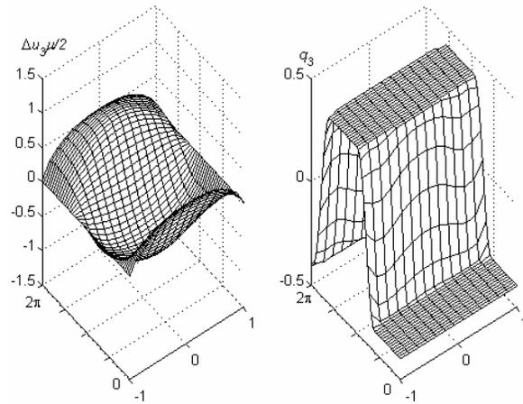
Figure 11: Crack opening and friction contact force for  $k_2 = 1.0$  and  $k_\tau = 0.4$ .
