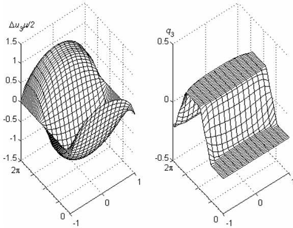
Figure 8: Crack opening and friction contact force for  $k_2 = 0.25$  and  $k_\tau = 0.2$ .
