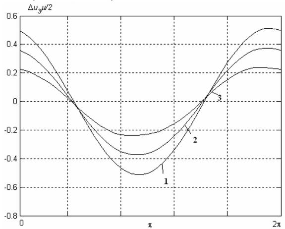
Figure 6: Crack opening  $k_2 = 1.75$ :  $1 - k_\tau = 0$ ,  $2 - k_\tau = 0.2$ ,  $3 - k_\tau = 0.4$ .
