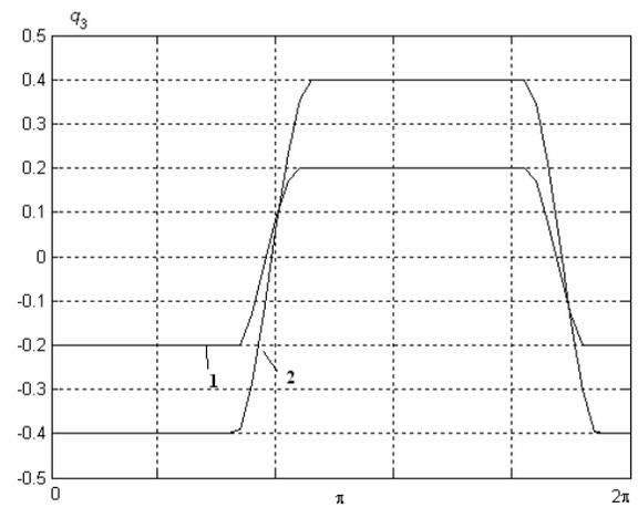
Figure 5: Friction contact force for  $k_2 = 1.0$ :  $1 - k_\tau = 0.2$ ,  $2 - k_\tau = 0.4$ .
