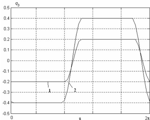
Figure 7: Friction contact force for  $k_2 = 1.75$ :  $1 - k_\tau = 0.2$ ,  $2 - k_\tau = 0.4$ .
