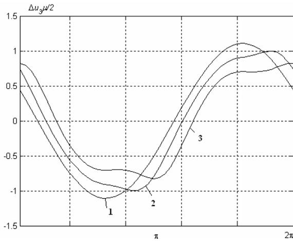
Figure 2: Crack opening  $k_2 = 0.25$ :  $1 - k_\tau = 0$ ,  $2 - k_\tau = 0.2$ ,  $3 - k_\tau = 0.4$ .
