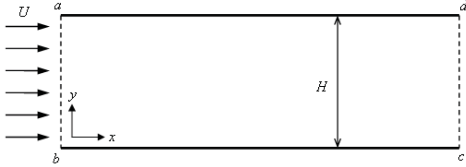
Figure 2: The simulation case (1) of channel flow without any build-in obstacles.
