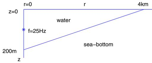
Figure 1: Benchmark wedge problem with a penetrable sea-bottom.
