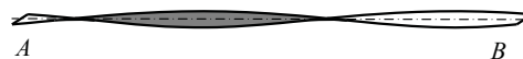
(a) A twisted ribbon with Wr=0, Tw=1 as shown in figure 9(a)
