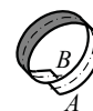
(b) A coiled ribbon with Wr \cong 0.95, Tw \cong 0.05 as shown in figure 9(e)
