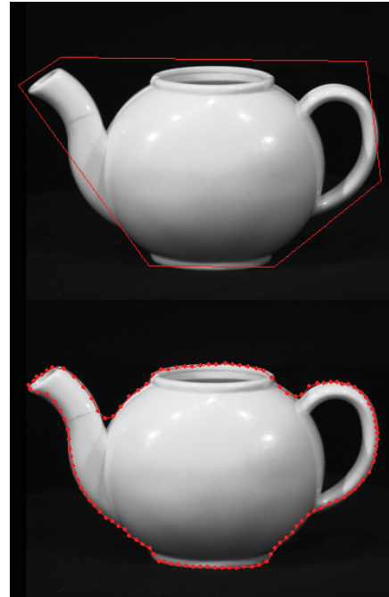
Figure 6: Initial contour defined further away from the object (top); result of the segmentation process using r=2,000\text{N/m} and a rubber model (bottom).
