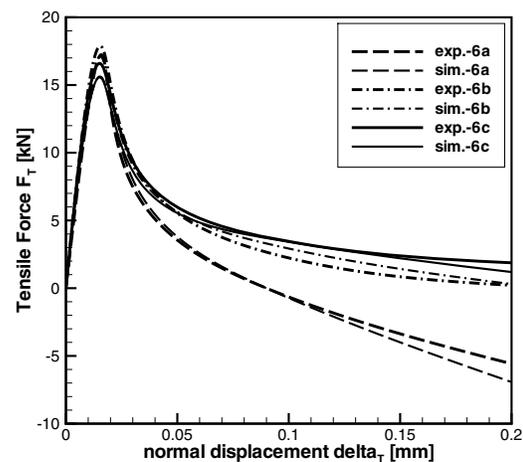
Figure 6: Tensile Force-displacement curve of the Nooru-Mohamed test for different load paths: 6a, 6b, 6c
