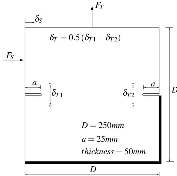
Figure 2: Nooru-Mohamed test: experimental set-up
