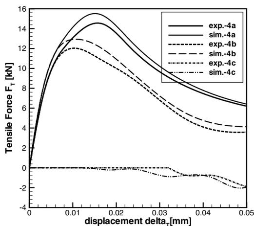
Figure 4: Tensile Force-displacement curve of the Nooru-Mohamed test for different load paths: 4a, 4b, 4c
