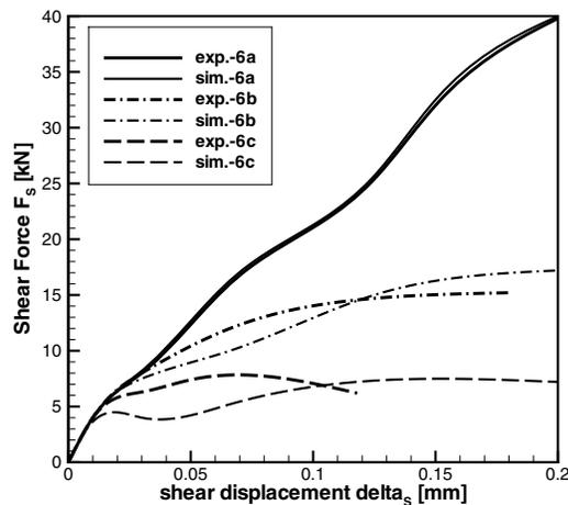
Figure 7: Shear Force-displacement curve of the Nooru-Mohamed test for different load paths: 6a, 6b, 6c
