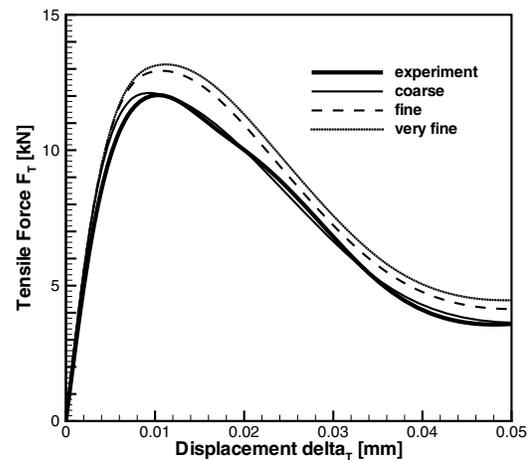
Figure 5: Mesh refinement study for specimen 4b
