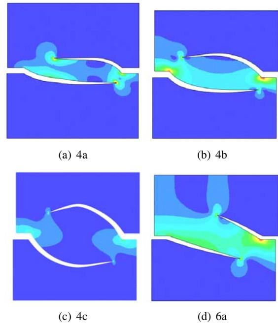
Figure 3: von Mises stress at the deformed specimen at failure of the Nooru-Mohamed test for different load paths
