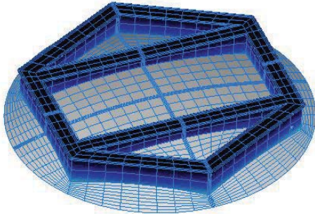
Figure 4: Finite element model for the reflector
