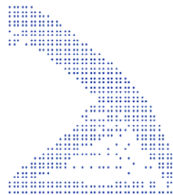
(c) Optimization result by RPIM with the densities of the Gauss quadrature points as a design variable
