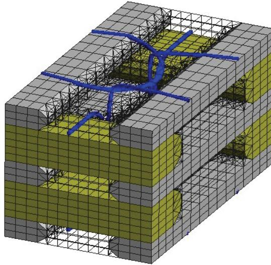
Figure 9: FE-mesh of a unit cell representing a textile reinforced composite
