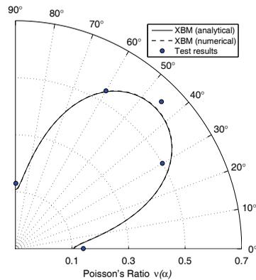
Figure 13: Polar diagram of in-plane Poisson's ratio
