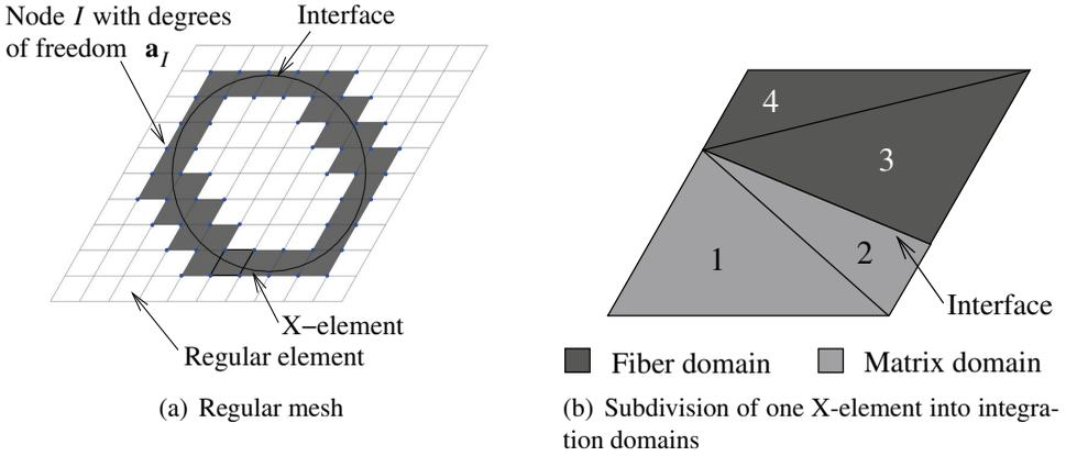
Figure 4: Model generation based on the X-FEM
