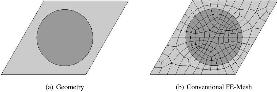
Figure 3: Unit cell of a UD-composite
