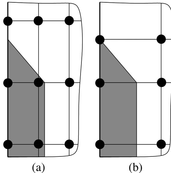
Figure 8: Modification of (a) element sizes and (b) location of element boundaries to avoid incompatible boundary conditions
