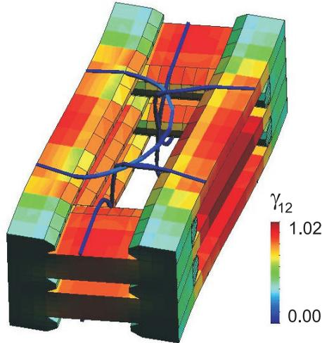
Figure 11: Deformation  $E_{12} = 1$  of the unit cell
