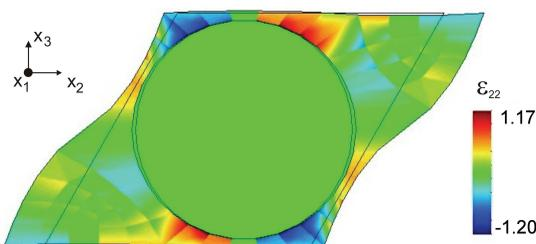
Figure 10: Deformation  $E_{22} = 1$  of a microscopic unit cell with  $v_W = 60\%$
