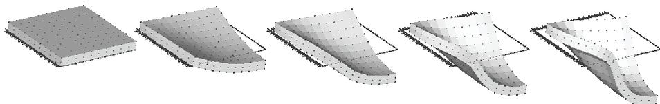
Figure 19: Deformation of the simply supported square plate for several increasing load levels.
