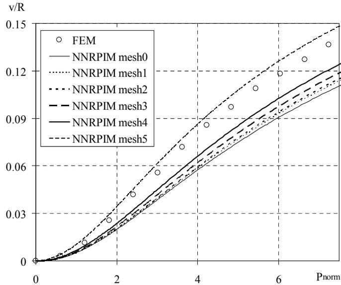
Figure 26: Evolution of the displacement along y direction on the end tip of the curved cantilever beam with the load level, for distinct meshes.
