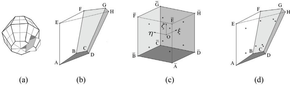
Figure 2: (a) Voronoi cell and respective tetrahedrons. (b) Initial tetrahedron. (c) Initial tetrahedron isoparameterization and determination of the quadrature integration points. (d) Quadrature integration points in Cartesian coordinates.
