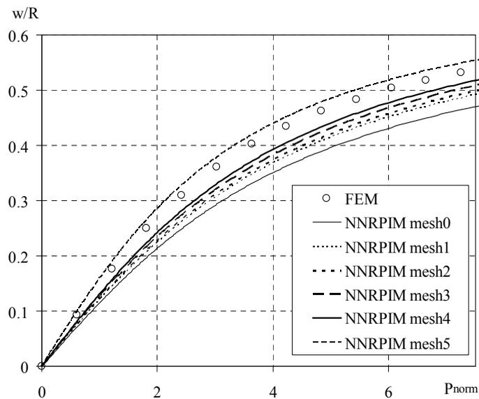
Figure 27: Evolution of the displacement along z direction on the end tip of the curved cantilever beam with the load level, for distinct meshes.
