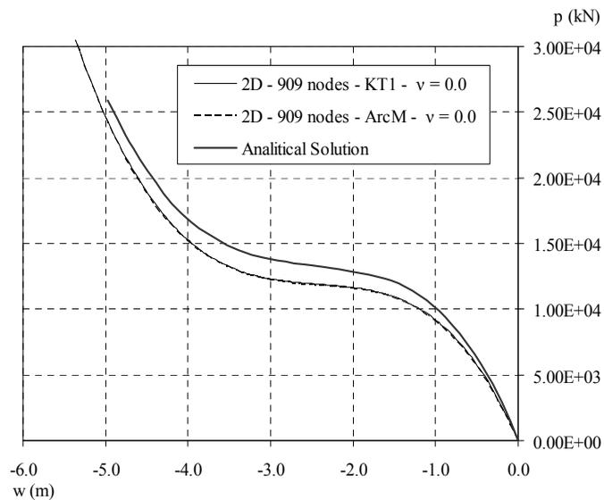
Figure 7: Evolution of the displacement on the mid span of the arch when two distinct non-linear solution methods are used.
