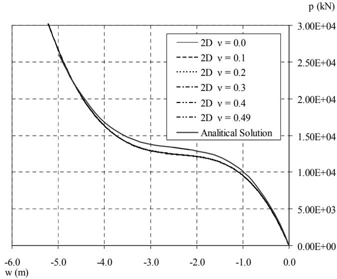
Figure 8: Evolution of the displacement on the mid span of the arch for several values of the Poisson ratio.
