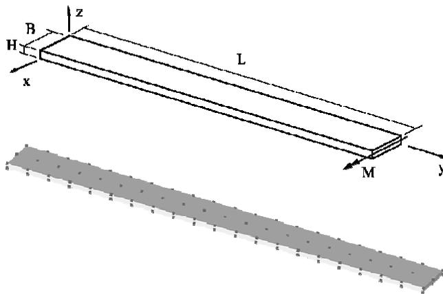
Figure 13: Geometrical model of the roll-beam proposed and Mesh used in the 3D analysis.
