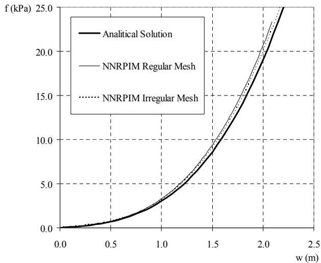
Figure 22: Central displacement of the plate in relation to the applied load for the 3D analysis.
