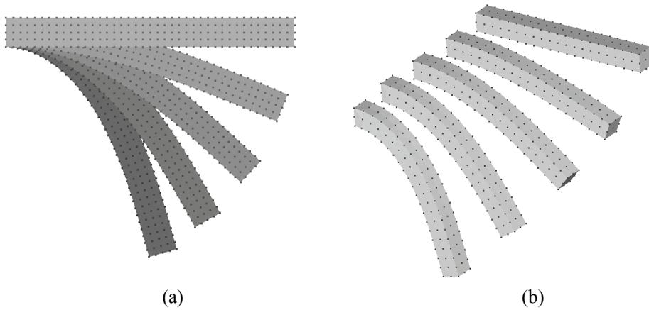
Figure 17: Deformation of the cantilever beam for several increasing load levels for the 2D analysis (a) and 3D analysis (b).
