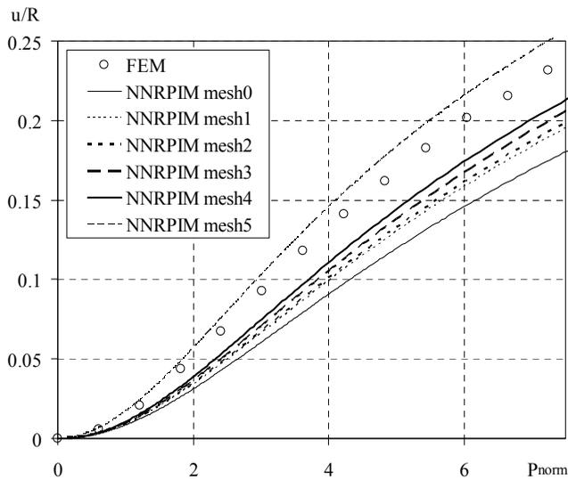
Figure 25: Evolution of the displacement along x direction on the end tip of the curved cantilever beam with the load level, for distinct meshes.
