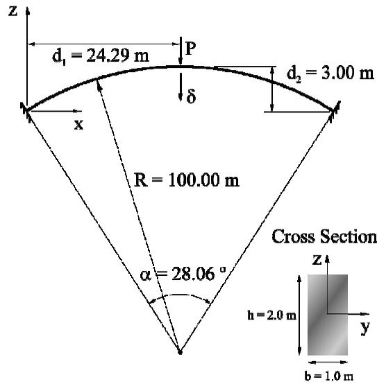
Figure 4: Geometrical model of proposed thick arch.
