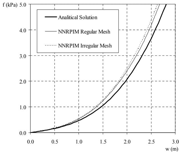
Figure 20: Evolution of the central displacement of the plate with the load level, for the 3D analysis.
