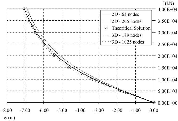
Figure 16: Evolution of the displacement on point A with the load level for distinct meshes, for the 2D and the 3D analysis.
