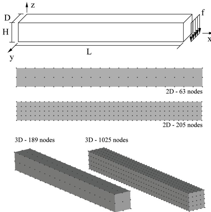
Figure 15: Geometrical model of the cantilever beam proposed and meshes considered in the analysis.
