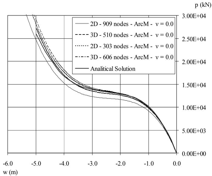
Figure 9: Evolution of the displacement on the mid span of the arch obtained with a 3D formulation and with irregular meshes.
