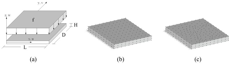
Figure 18: (a) Geometrical model of the plate and applied load. (b) Regular mesh with 363 nodes and (c) Irregular mesh with 474 nodes.
