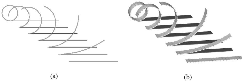
Figure 14: Deformed meshes for increasing tip moments for the 2D analysis (a) and the 3D analysis (b).
