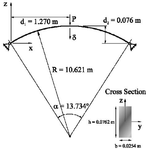
Figure 10: Geometrical model of the proposed shallow arch.
