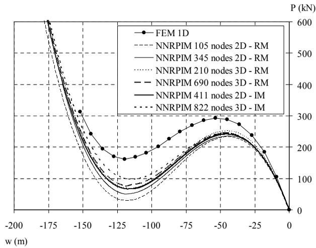
Figure 12: Displacement on the mid span of the arch.
