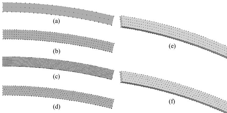
Figure 5: Meshes used in the analysis. (a) 2D regular 73 nodal mesh. (b) 2D regular 255 nodal mesh. (c) 2D regular 909 nodal mesh. (d) 2D irregular 303 nodal mesh. (e) 3D regular 510 nodal mesh. (f) 3D irregular 606 nodal mesh.
