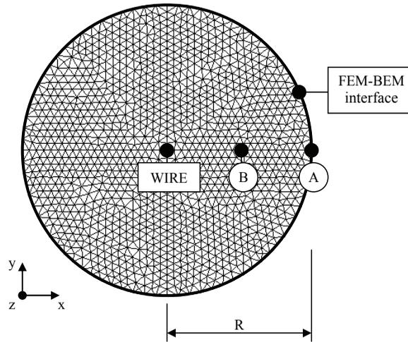
Figure 2: Sketch of the infinite domain model: circular FEM-BEM interface enclosing the FEM sub-domain and the centrally located wire.
