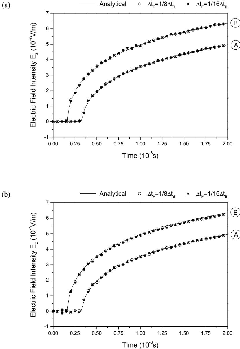
Figure 3: Time-history results for the electric field intensity at points A and B considering FEM-BEM coupled analyses and different temporal discretizations for each sub-domain: (a) algorithm 1; (b) algorithm 2.
