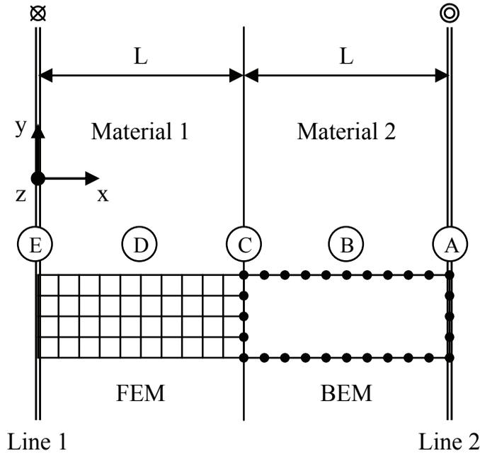
Figure 4: Sketch of the finite domain model: opposite lines of wires and sub-domains spatial discretizations.
