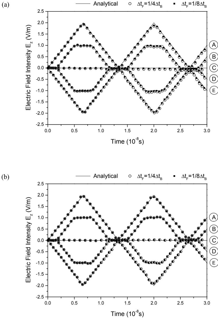
Figure 5: Time-history results for the electric field intensity at points A, B, C, D and E considering FEM-BEM coupled analyses and different temporal discretizations for each sub-domain (air-air model): (a) algorithm 1; (b) algorithm 2.
