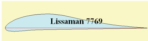
Figure 1: Lissaman 7769 airfoil geometry
