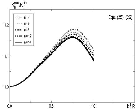
Figure 4: Stress intensity factor (the transverse shear mode) plotted against the wave number,  $\rho^{(1)} = \rho^{(2)}$ ,  $\mu^{(1)} = 2\mu^{(2)}$
