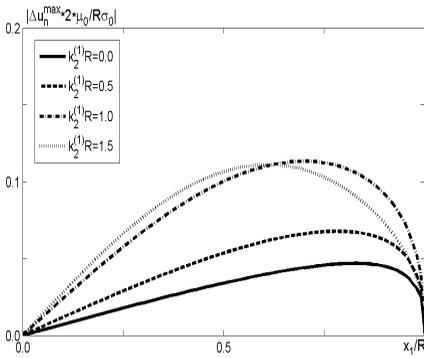
Figure 1: Normal displacement discontinuity at the crack surface,  $\rho^{(1)} = \rho^{(2)}$ ,  $\mu^{(1)} = 2\mu^{(2)}$
