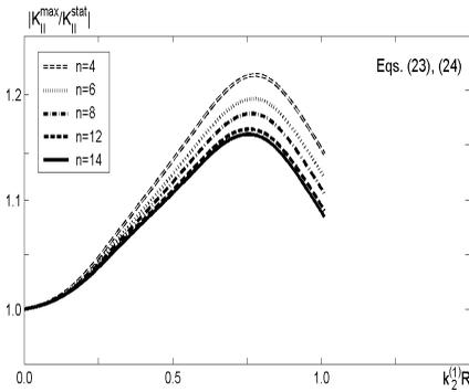
Figure 3: Stress intensity factor (the transverse shear mode) plotted against the wave number,  $\rho^{(1)} = \rho^{(2)}$ ,  $\mu^{(1)} = 2\mu^{(2)}$
