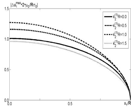
Figure 2: Tangential displacement discontinuity at the crack surface,  $\rho^{(1)} = \rho^{(2)}$ ,  $\mu^{(1)} = 2\mu^{(2)}$
