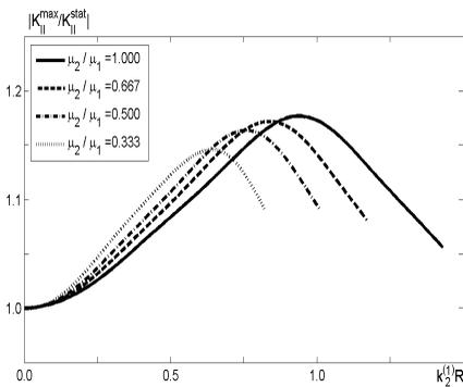
Figure 7: Stress intensity factor (transverse shear mode) plotted against the wave number,  $\rho^{(1)} = \rho^{(2)}$ ,  $\mu^{(2)}/\mu^{(1)} < 1$
