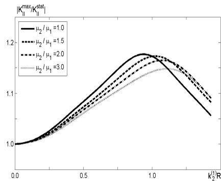
Figure 8: Stress intensity factor (transverse shear mode) plotted against the wave number,  $\rho^{(1)} = \rho^{(2)}$ ,  $\mu^{(2)}/\mu^{(1)} > 1$
