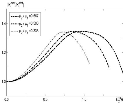
Figure 5: Stress intensity factor (the opening mode) plotted against the wave number,  $\rho^{(1)} = \rho^{(2)}$ ,  $\mu^{(2)}/\mu^{(1)} < 1$
