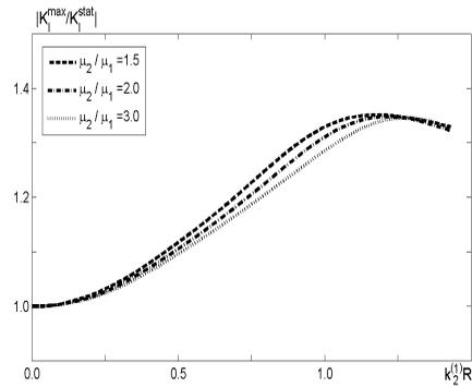
Figure 6: Stress intensity factor (the opening mode) plotted against the wave number,  $\rho^{(1)} = \rho^{(2)}$ ,  $\mu^{(2)}/\mu^{(1)} > 1$
