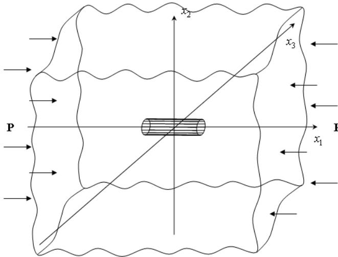
Figure 1: Model of composite reinforced by nanotube
