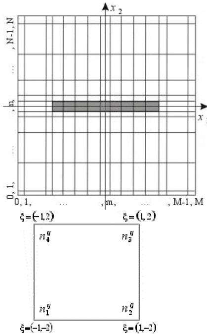
Figure 3: Calculation scheme of nanocomposite
