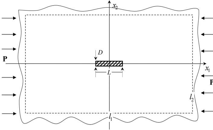
Figure 2: Plane model of nanocomposite
