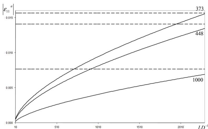
Figure 4: Dependence of the value of critical strain for a fiber on the geometrical parameters of fibers
