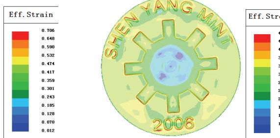
Figure 20: Effective stress contour of the first layer elements
