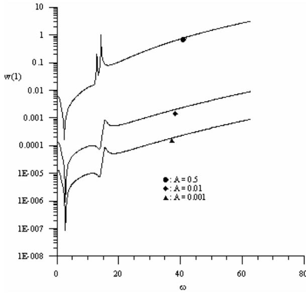
Figure 5: Influence of the excitation frequency  $\omega$  and the amplitude of excitation angle  $A$  on the tip amplitude of an inward rotating beam. [ $r_0=1, m_{tip} = 100, C = 1$ ].
