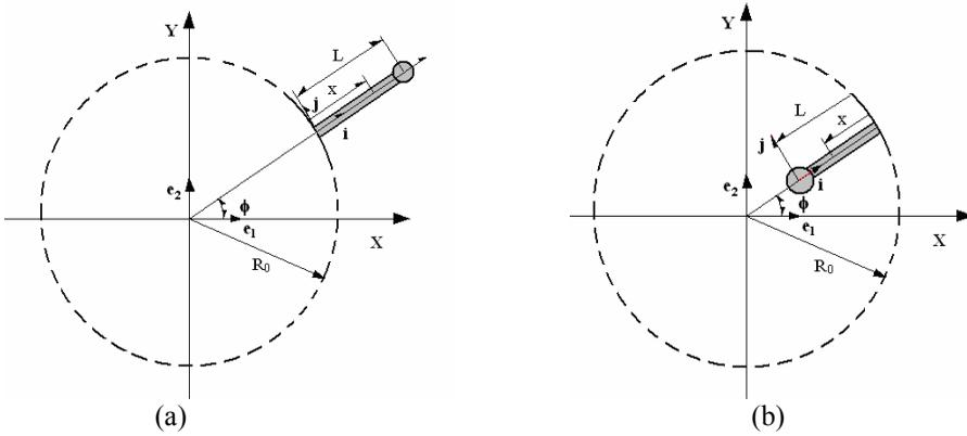
Figure 1: Geometry and coordinate system of a moving beam with a tip mass.
