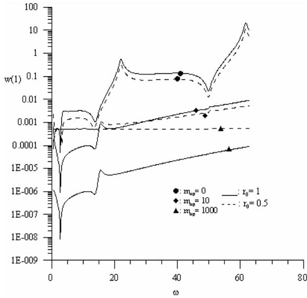
Figure 2: Influence of the excitation frequency  $\omega$ , the tip mass  $m_{tip}$  and the root radius  $r_0$  on the tip amplitude of an inward rotating beam. [A = 0.001, C = 1].
