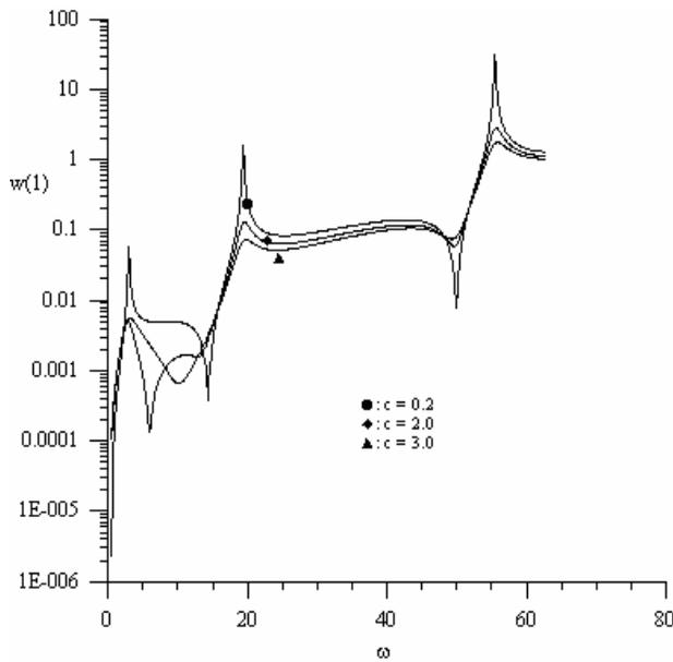
Figure 6: Influence of the excitation frequency  $\omega$  and the damping constant  $c$  on the tip amplitude of an inward rotating beam. [ $r_0=1.5, m_{tip} = 0.1, A = 0.001$ ].
