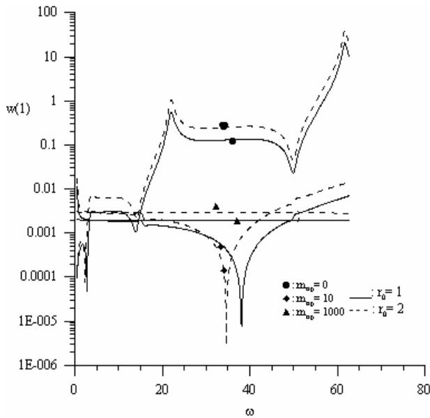
Figure 3: Influence of the excitation frequency  $\omega$ , the tip mass  $m_{tip}$  and the root radius  $r_0$  on the tip amplitude of an outward rotating beam. [A = 0.001, C = 1].
