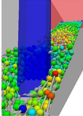
Figure 5: Debris deflection at the single-column barrier
