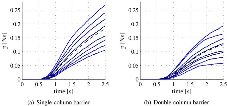
Figure 7: Uncertain accumulated impulse over time for two debris-flow barrier designs.
