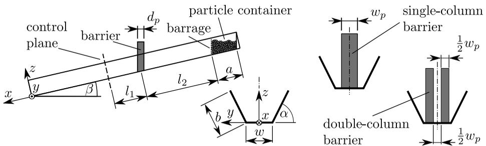
Figure 3: Setup of the chute flow laboratory model.
