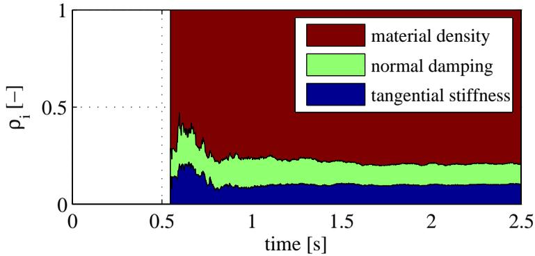
Figure 8: Normalized relative measure of influence  $\rho_i$  for the accumulated impulse on the control plane behind the single-column barrier.
