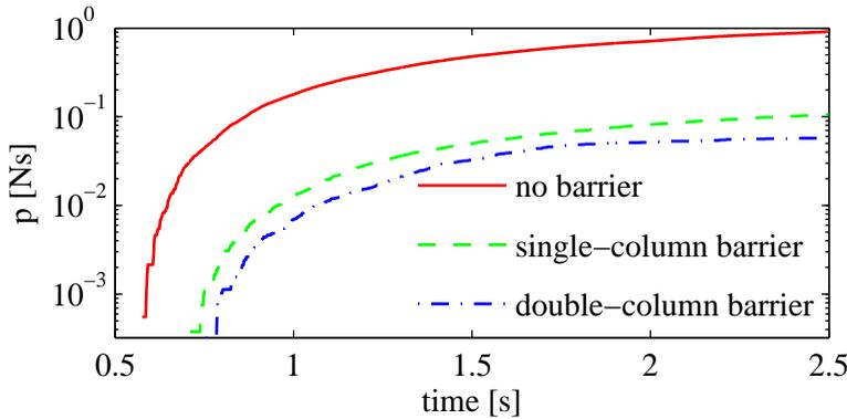
Figure 6: Accumulated impulse on the control plane for the nominal input parameter set.
