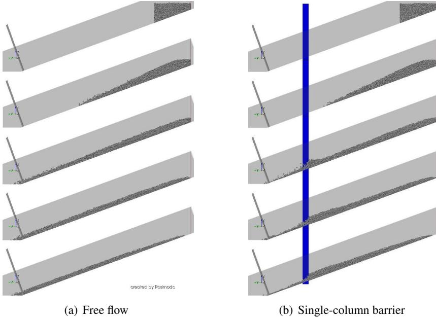
Figure 4: Snapshots from chute flow particle simulations.
