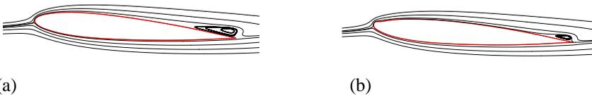
Figure 16: Minimization of  $\overline{C_d}$  at  $Re = 10^3$  and  $\alpha = 5^\circ$ : time-averaged streamlines for (a) NACA 0012 (b) optimal shape.
