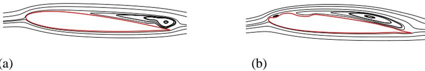
Figure 30: Minimization of  $\overline{C_d}/\overline{C_l}$  at  $Re = 10^4$  and  $\alpha = 5^\circ$ : time-averaged streamlines for (a) NACA 0012 (b) optimal shape.
