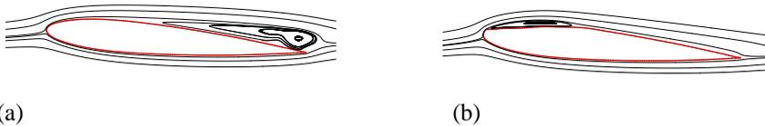
Figure 21: Minimization of  $\overline{C_d}$  at  $Re = 10^4$  and  $\alpha = 5^\circ$ : time-averaged streamlines for (a) NACA 0012 (b) optimal shape.
