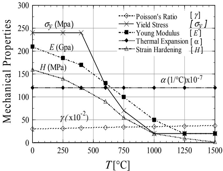
Figure 2: Mechanical properties of mild steel
