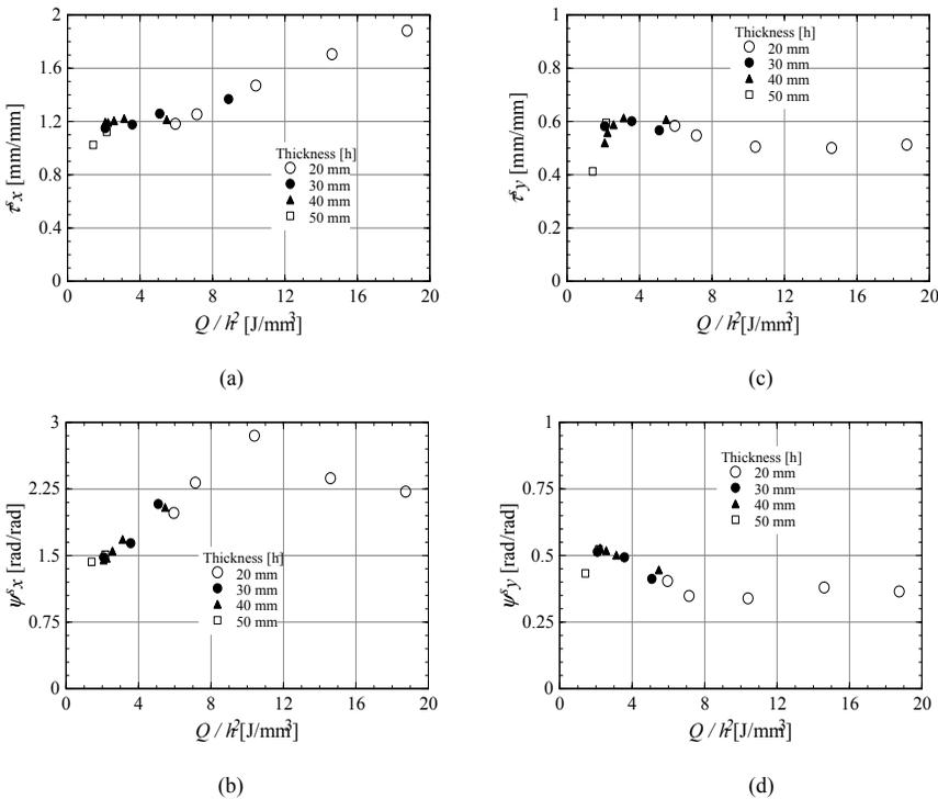
Figure 13: Relation between edge effect and heat input parameter  $Q/h^2$  at the entrance plate edge (a) Longitudinal shrinkage, (b) Transverse shrinkage, (c) Longitudinal bending and (d) Transverse bending
