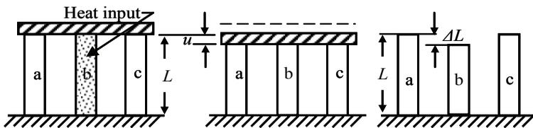
Figure 5: Mechanical model used to analyze the longitudinal components of inherent deformation
