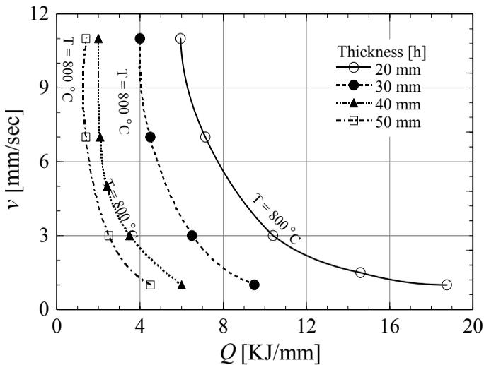
Figure 7: Relationship between heat input and speed of the heating source
