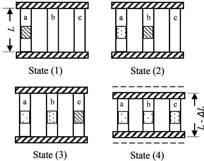
Figure 4: Mechanical model used to analyze the transverse component of inherent deformation
