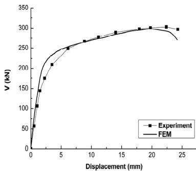
Figure 6: Shear force-displacement curve
