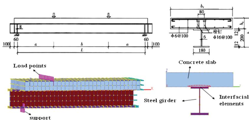
Figure 2: Features of the continuous beam and the 1/2 FE model
