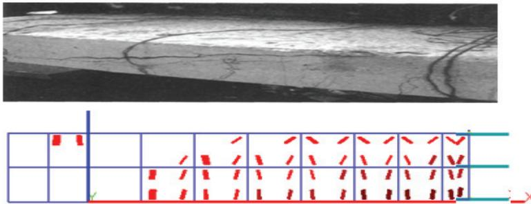
Figure 8: Crack pattern compared with the experimental results
