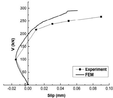
Figure 7: Shear force-slip curve
