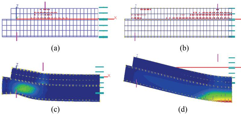
Figure 4: Crack pattern at the ultimate load (a): CBS-9 (b): CBS-12 displacement and contour at the ultimate load (c) : CBS-9 (d): CBS-12
