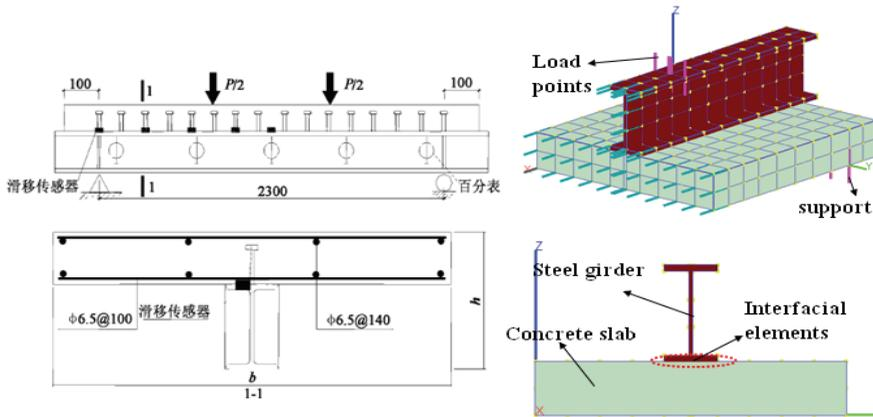
Figure 5: Features of the composite beam and the 1/2 FE model
