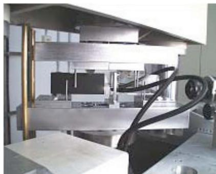
Figure 31: Four point bending test.
