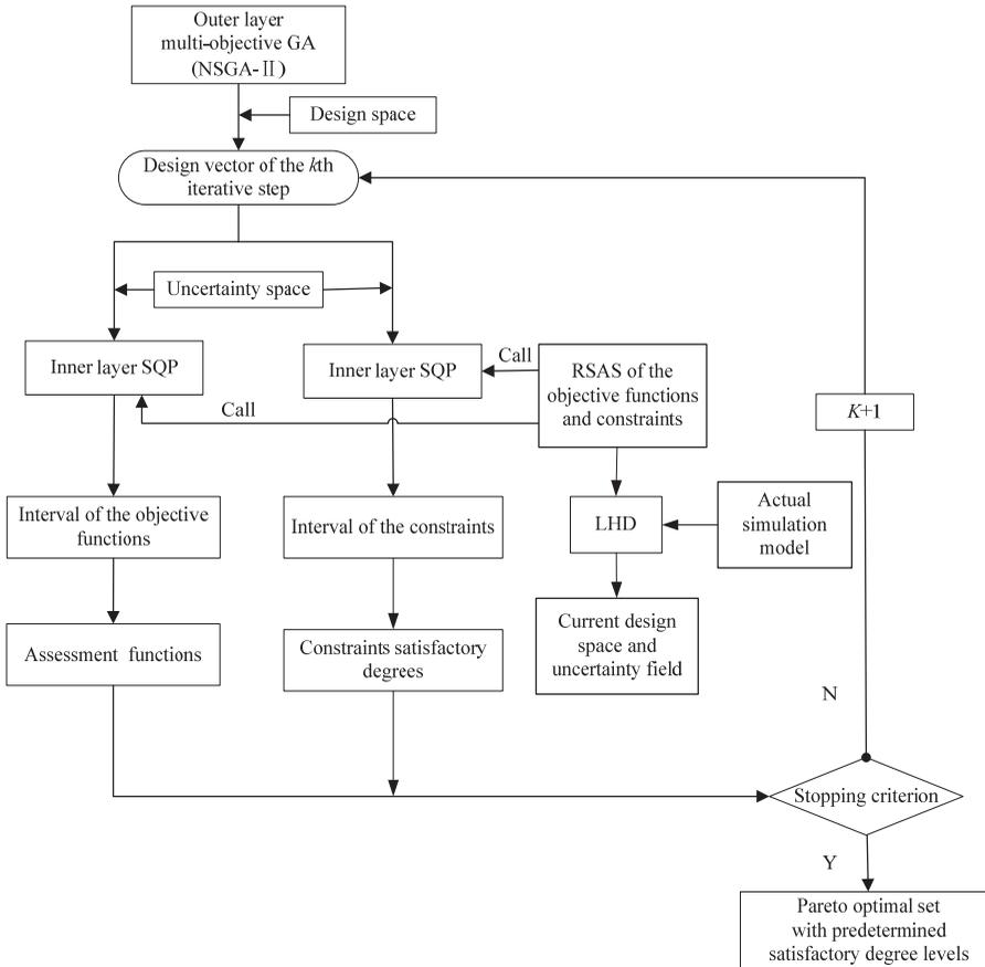
Figure 2: Flowchart of the present method nesting optimization based on the actual simulation models
