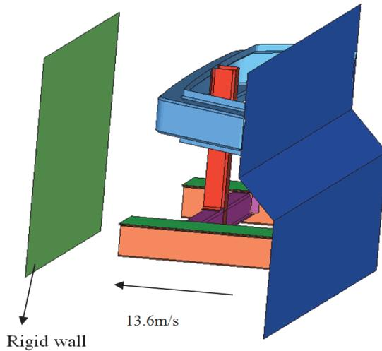
Figure 6: A bumper impacting the rigid wall
