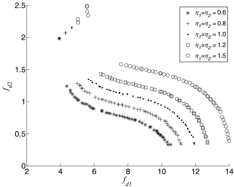
Figure 3: The Pareto optimal fronts with different satisfactory degree levels
