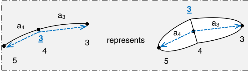
Figure 2: Representation of two semicracks that compose the crack element # 3 related to node # 4.
