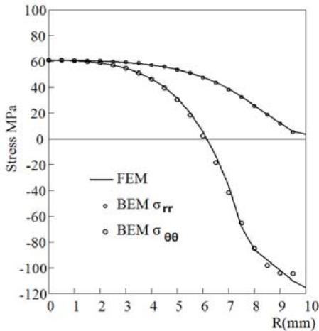
Figure 3: Thermal stress distribution (plane stress)
