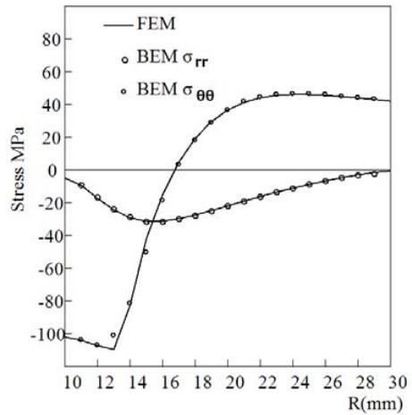
Figure 6: Thermal stress distribution (plane stress)
