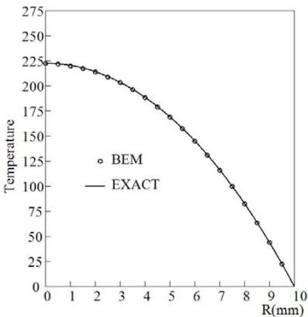
Figure 7: Temperature distribution in a circular region
