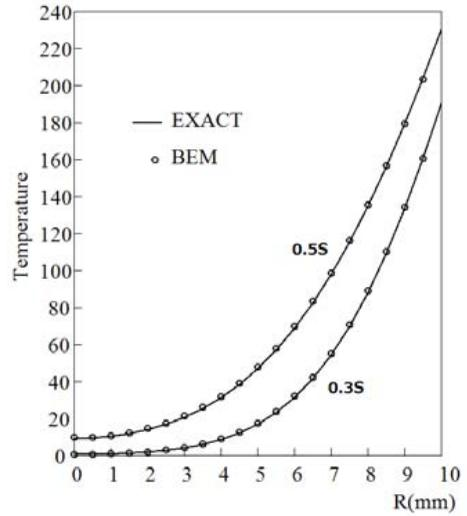
Figure 2: Temperature distribution in a circular region
