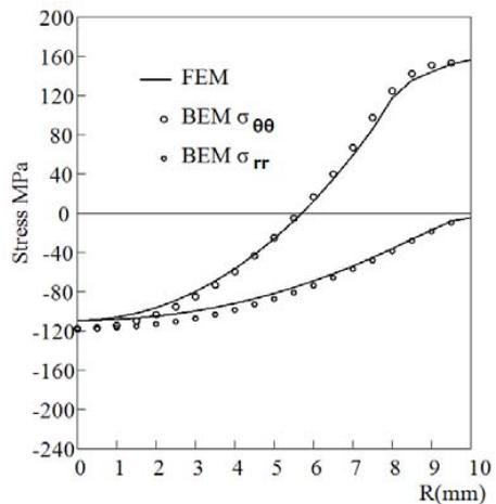
Figure 8: Thermal stress distribution with heat generation (plane stress)
