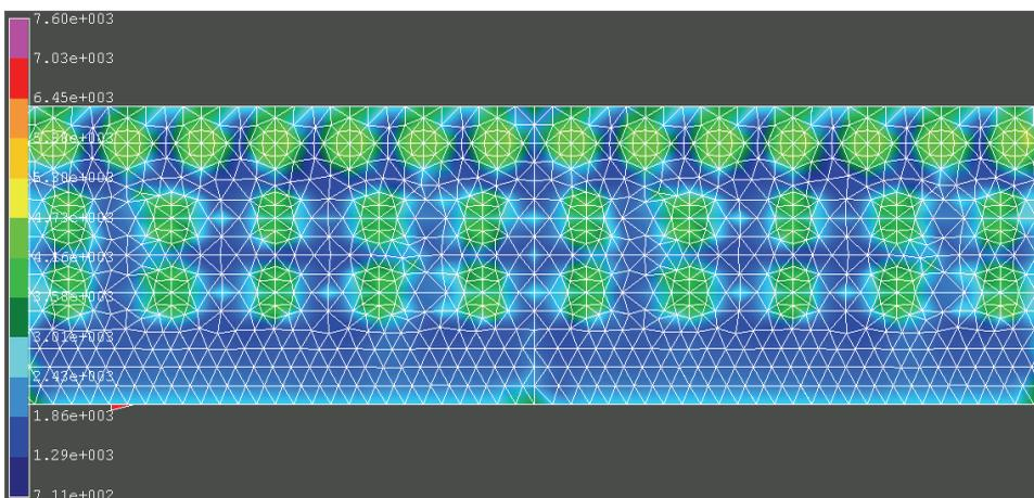
Figure 15: Normal stress distribution of the tensile direction ( $\sigma_{xx}$ ) of the specimen
