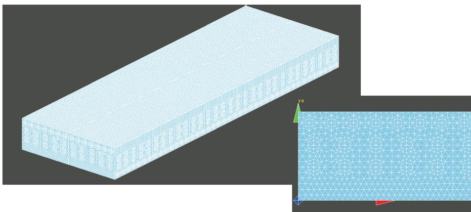
Figure 14: Finite element mesh of the specimen of the woven composite plate
