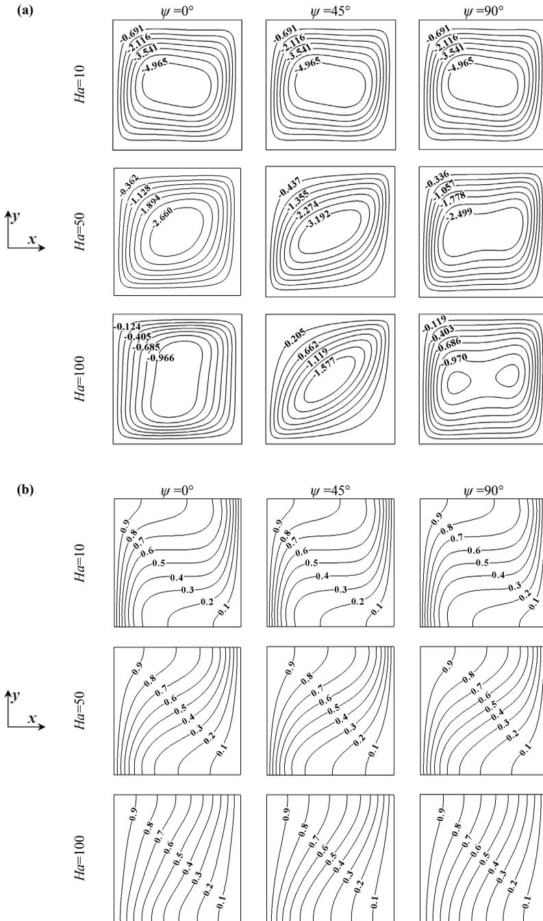
Figure 10: Dynamic (a) and thermal (b) structures for  $Ra=10^5$ ,  $\phi=0^\circ$ ,  $Pr=1$ ,  $Da=10^{-2}$  and  $\epsilon=0.4$
