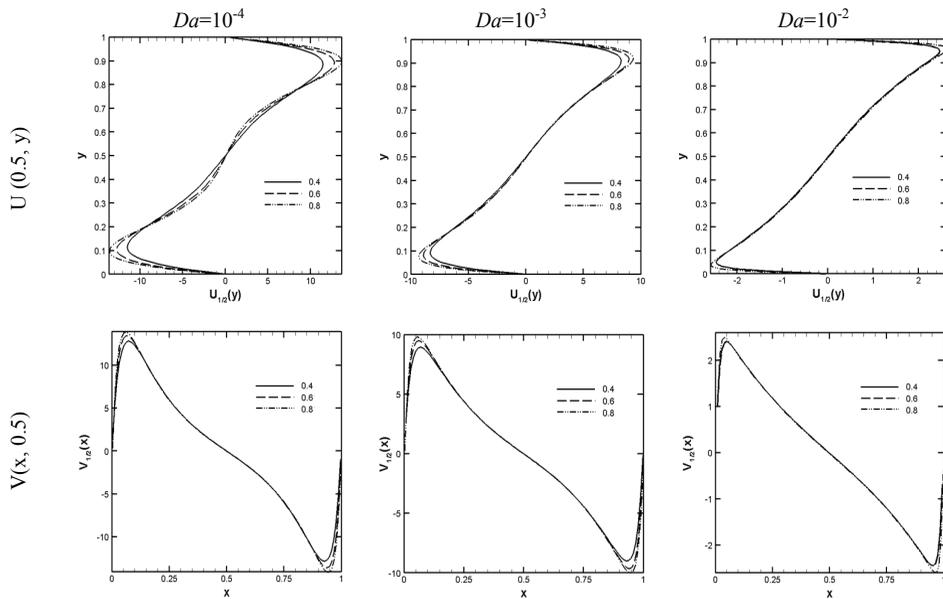
Figure 6: Velocities profiles at the horizontal and vertical mid-planes for different Darcy numbers and medium porosities for  $Ra=10^5$ ,  $\varphi=0^\circ$ , and  $Ha=50$ .
