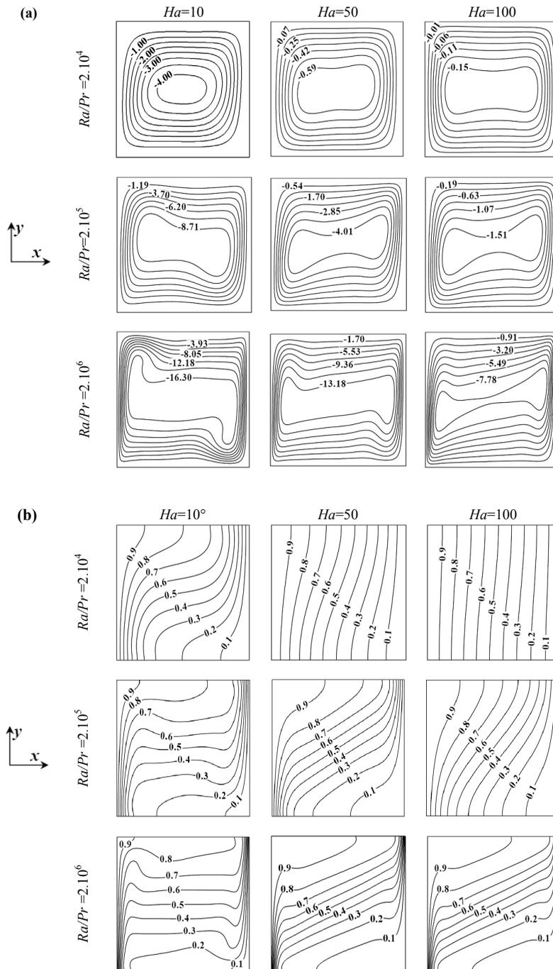
Figure 3: Dynamic (a) and thermal (b) structures for free fluid flow for  $Pr=0.733$  and  $\phi=0^\circ$
