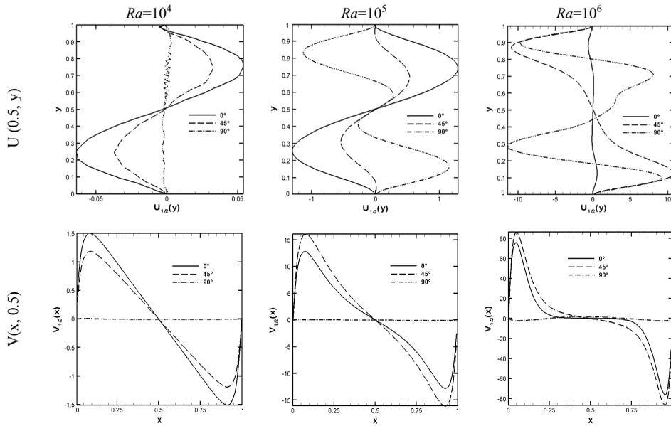
Figure 5: Velocities profiles at the horizontal and vertical mid-planes for different Rayleigh numbers and cavity inclinations for  $Da=10^{-2}$ ,  $\varepsilon=0.4$ , and  $Ha=50$ .
