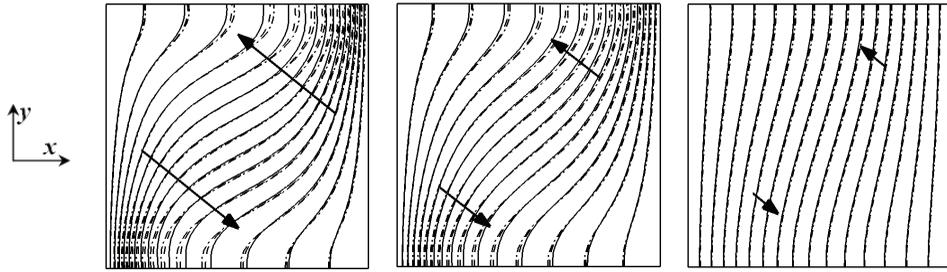
Figure 8: Effect of the Darcy number on thermal structure for  $Da=10^{-4}$ ,  $10^{-3}$  and  $10^{-2}$  (from left to right). For  $Ra=10^5$ ,  $\phi=0^\circ$ ,  $Pr=1$ ,  $Ha=50$  and  $\psi=0^\circ$ .  $\varepsilon=0.4$ : solid line,  $\varepsilon=0.6$ : dashed line and  $\varepsilon=0.8$ : dash-dotted line.
