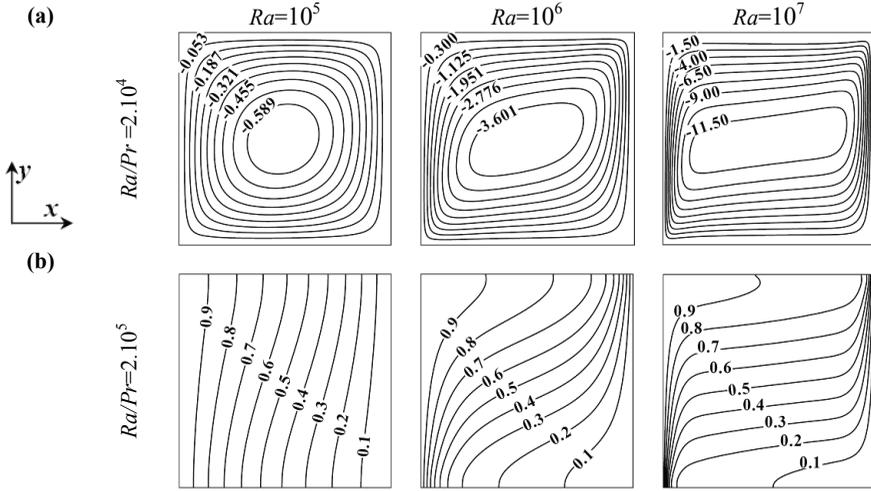
Figure 2: Dynamic (a) and thermal (b) structures for  $\epsilon=0.4, Pr=1, Da=10^{-4}$ .
