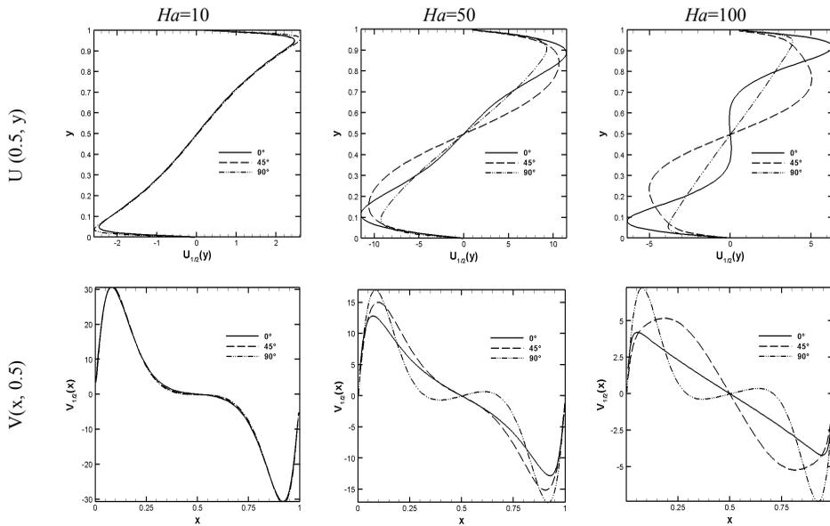
Figure 9: Velocities profiles at the horizontal and vertical mid-planes for different Hartmann numbers and magnetic field orientations for  $Ra=10^5$ ,  $\phi=0^\circ$ ,  $Da=10^{-2}$  and  $\varepsilon=0.4$ .
