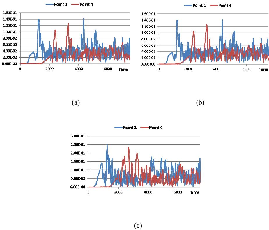
Figure 7: Displacement responses in optical mode along (a) x-axis, (b) y-axis, and (c) z-axis
