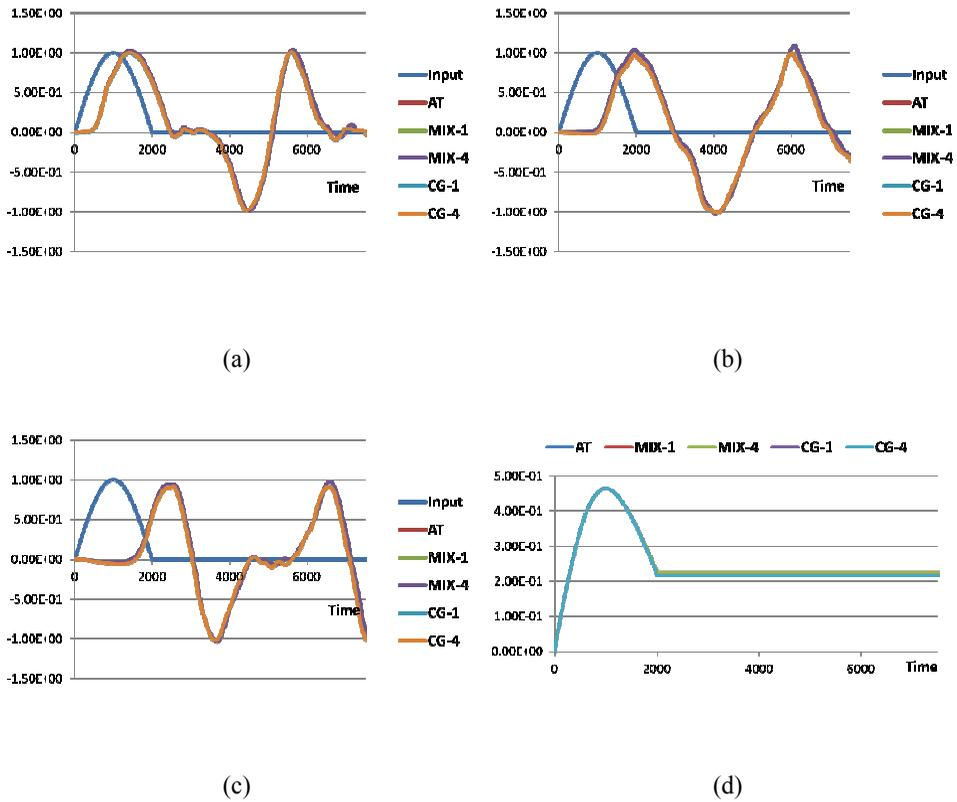
Figure 5: Displacement response of (a) Point 1, (b) Point 2, (c) Point 4 and (d) total energy
