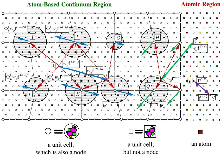
Figure 1: The schematic of multiple length scale modeling
