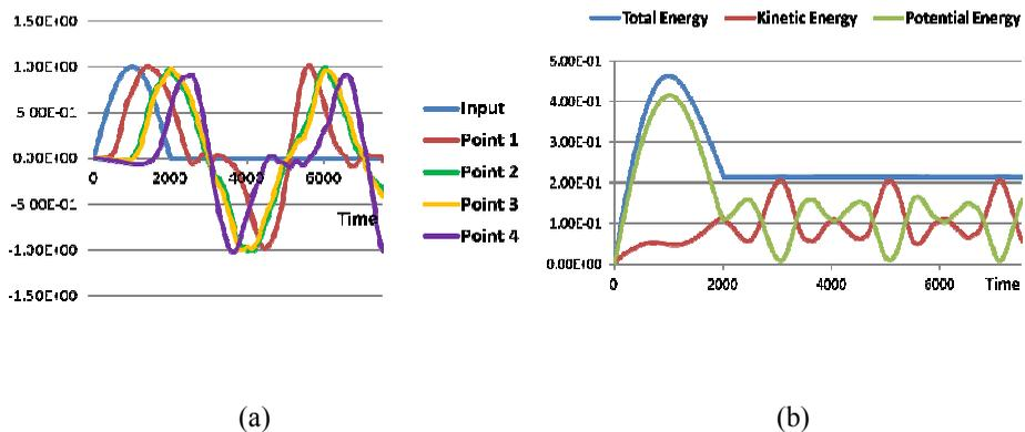
Figure 6: (a) Displacement responses in acoustic mode of Point 1, Point 2, Point 3 and Point 4; and (b) energies variations
