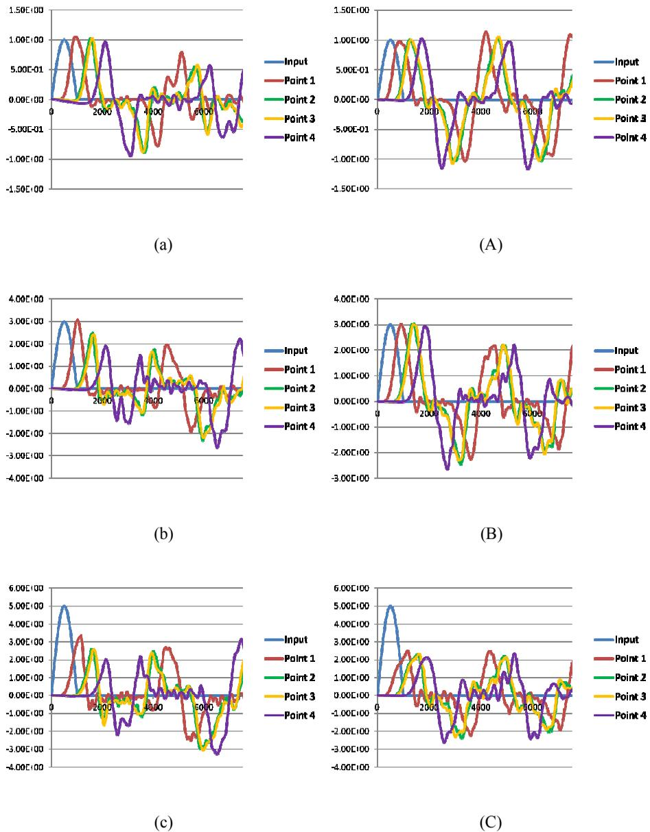
Figure 8: Displacement responses subject to impulse with magnitude equals to, (a) 1, (b) 3, and (c) 5
