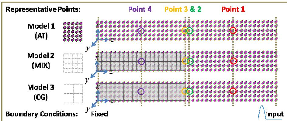
Figure 4: Computational models of a clamped MgO specimen under an impulsive loading and the positions of the selected representative points.
