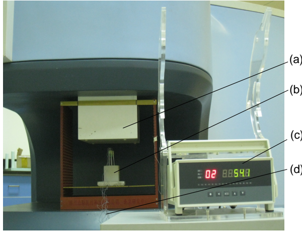
Figure 6: Schematic of the experiment (a)Magnetic pole, (b)Phantom, (c)Thermometer, (d)Thermocouple
