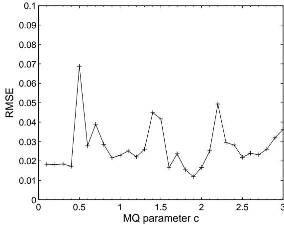
Figure 3: Effect of MQ parameter to numerical results.
