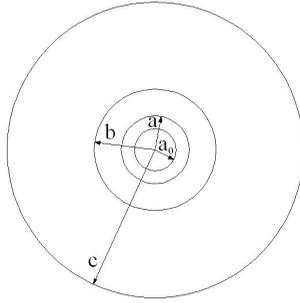
Figure 6: Casing-Cement-Formation System
