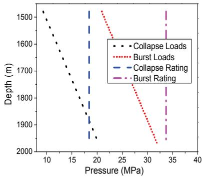
Figure 5: Casing strength check (40°)
