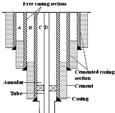
Figure 2: Schematic diagram of well structure
