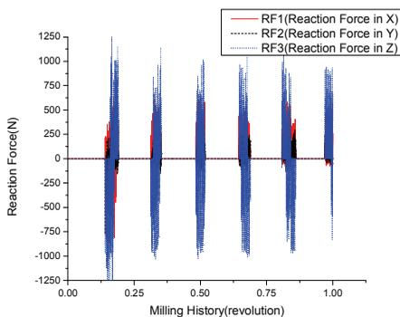
Figure 11: The reaction forces (FPR=0.9mm)
