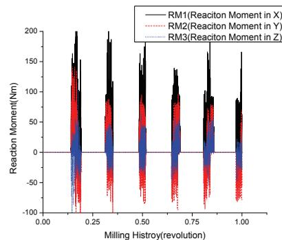
Figure 12: The reaction moments (FPR=0.9mm)
