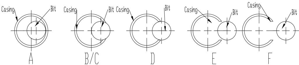
Figure 1: The process of casing window milling
