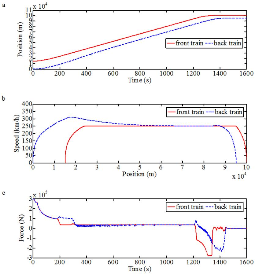
Figure 9: Train following process, updated trajectory and optimized tractive force. (a) position versus time, (b) speed versus position, and (c) tractive force.
