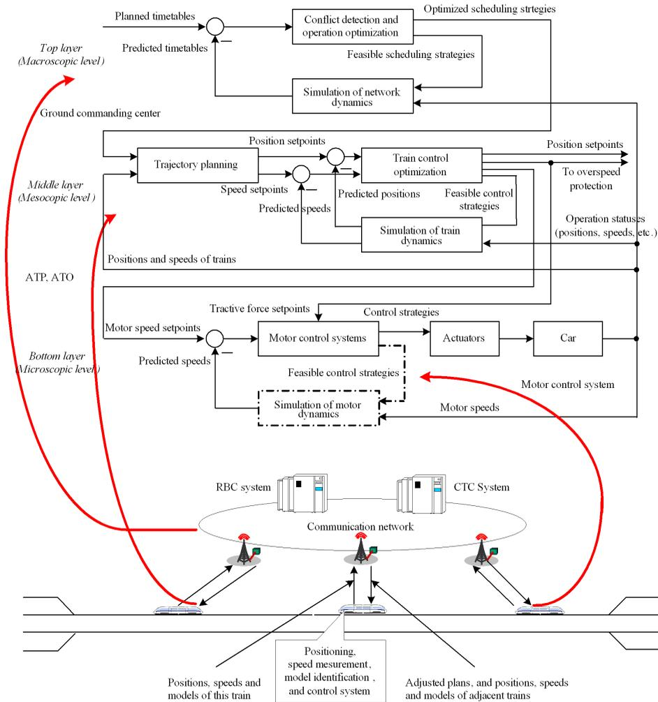
Figure 1: The hierarchical integration architecture of real-time train scheduling and control
