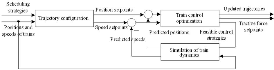
Figure 3: Basic framework of train operation planning based on MPC with automatic trajectory configuration
