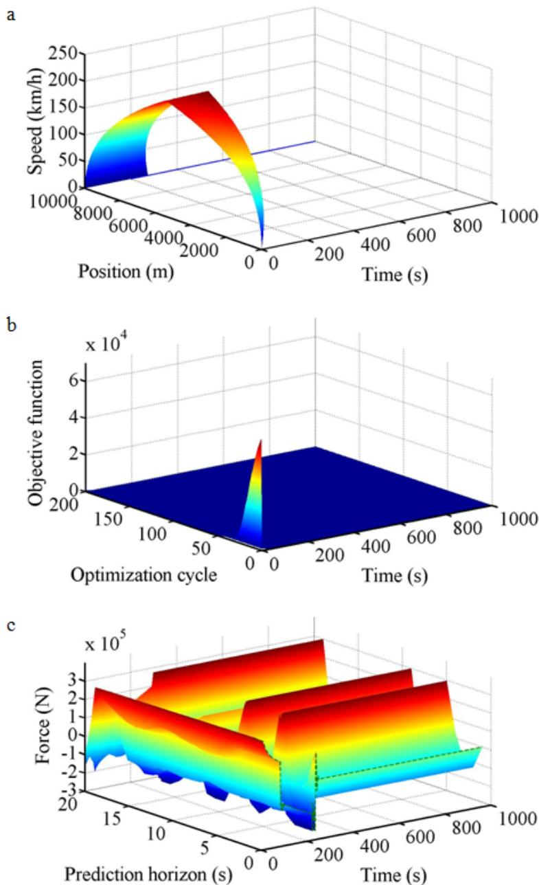
Figure 4: Optimization process of tractive force. (a) configured trajectory, (b) optimization process, and (c) tractive force.
