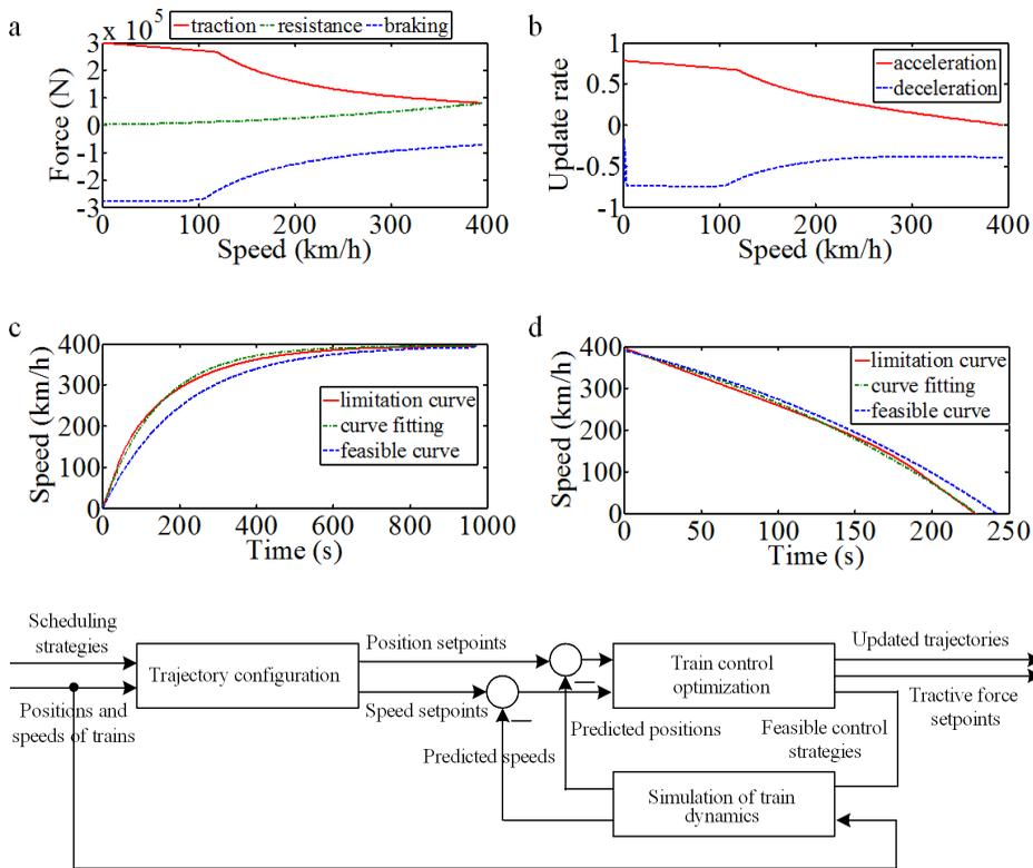
Figure 2: The curves required and engendered in automatic trajectory configuration. (a) tractive and braking forces, and basic resistance, (b) speed update rate, (c) acceleration process, (d) deceleration process, (e) acceleration distance, (f) deceleration distance, (g) configured trajectory 1, and (h) configured trajectory 2.
