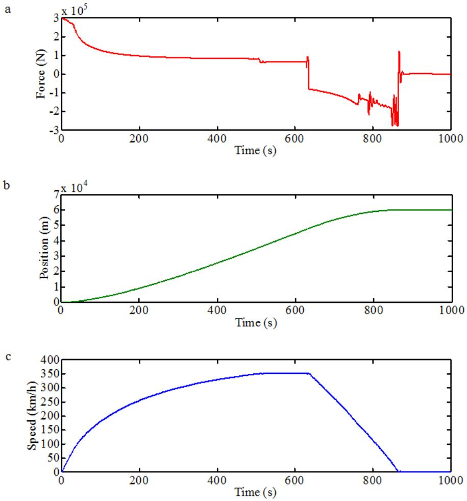
Figure 7: Optimized tractive force and updated trajectories. (a) tractive force, (b) position versus time, and (c) speed versus time.
