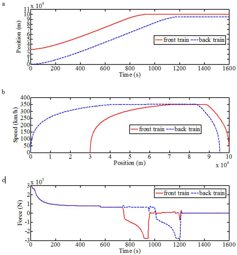
Figure 11: Train following process, updated trajectory and optimized tractive force. (a) position versus time, (b) speed versus position, and (c) tractive force.
