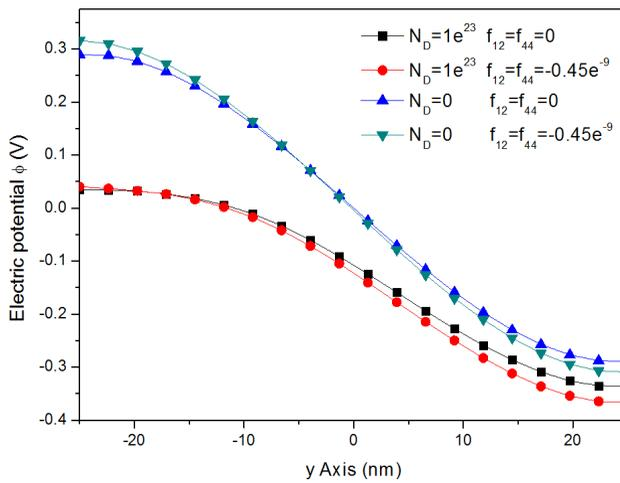
Figure 7: Electric potential along diameter with different donor concentration and flexoelectric constants
