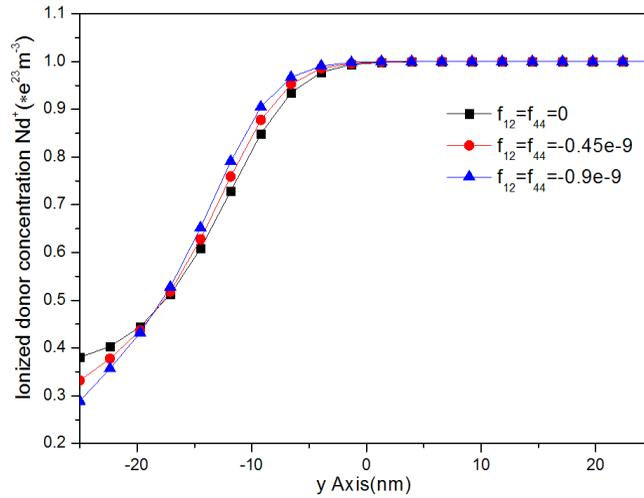
Figure 4: Line plot of  $N_D^+$  with different flexoelectric constants along the diameter
