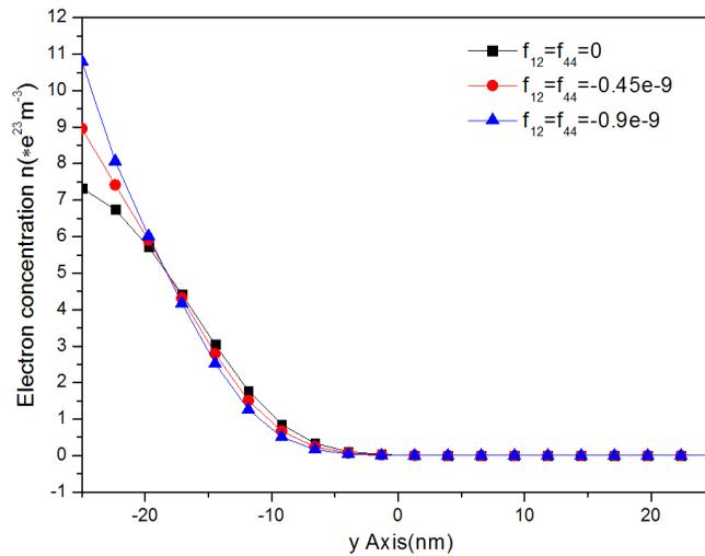
Figure 5: Line plot of  $n$  with different flexoelectric constants along the diameter
