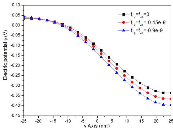
Figure 3: Line plot of  $\phi$  with different flexoelectric constants along the diameter
