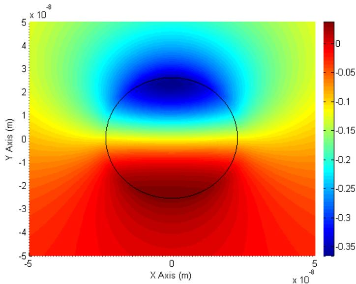
Figure 2: Cross section color plot of electric potential  $\phi$  considering the flexoelectric effect
