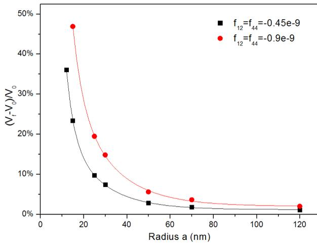
Figure 6: Values of  $(V_f - V_0)/V_0$  with radius
