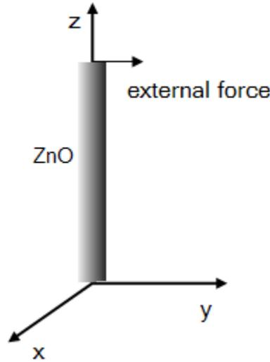
Figure 1: External force applied on the ZnO NW
